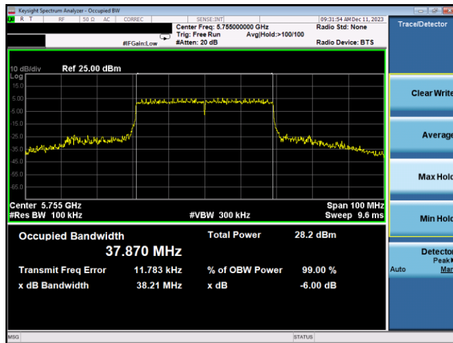
Plot 7-164. 6dB BW & 99% OBW Antenna 1b (40MHz BW 11ax – RU484 – Ch.151)
