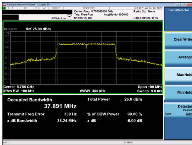
Plot 7-152. 6dB BW & 99% OBW Antenna 3a (40MHz BW 11ax – RU484 – Ch.151)
