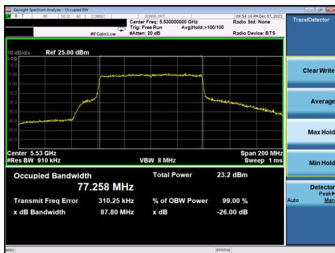
Plot 7-20. 26dB BW & 99% OBW Antenna 3c (80MHz BW 802.11ax(SU) – Ch. 106, MCS2)
