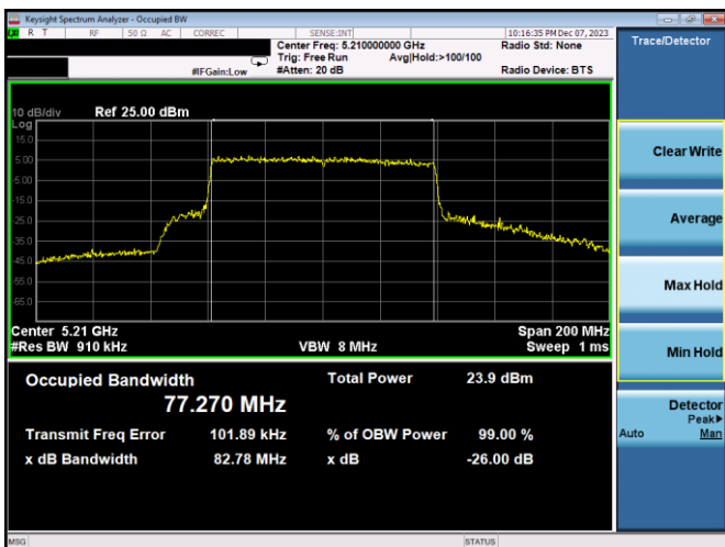
Plot 7-28. 26dB BW & 99% OBW Antenna 3c (80MHz BW 802.11ax(SU) – Ch. 42, MCS4)
