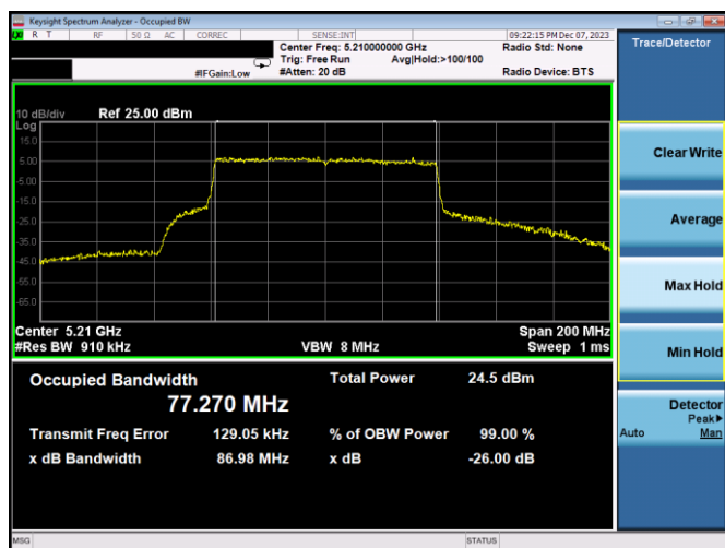
Plot 7-6. 26dB BW & 99% OBW Antenna 3c (80MHz BW 802.11ax(SU) – Ch. 42, MCS2)
