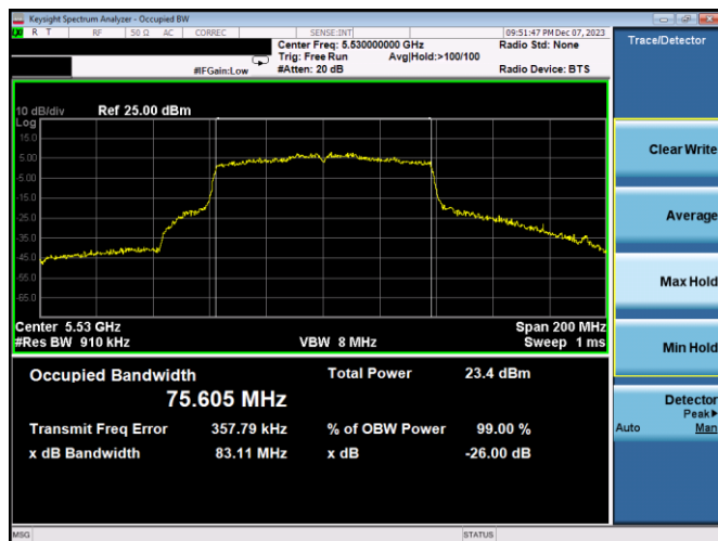
Plot 7-19. 26dB BW & 99% OBW Antenna 3c (80MHz BW 802.11ac – Ch. 106, MCS2)
