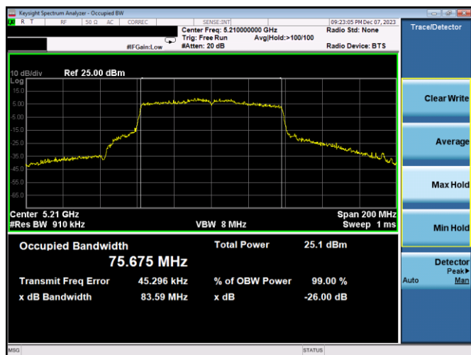
Plot 7-5. 26dB BW & 99% OBW Antenna 3c (80MHz BW 802.11ac – Ch. 42, MCS2)
