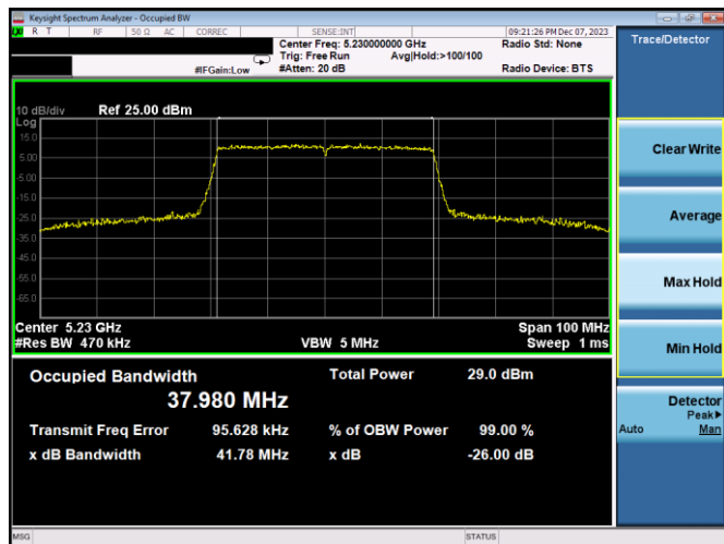
Plot 7-4. 26dB BW & 99% OBW Antenna 3c (40MHz BW 802.11ax(SU) – Ch. 46, MCS2)
