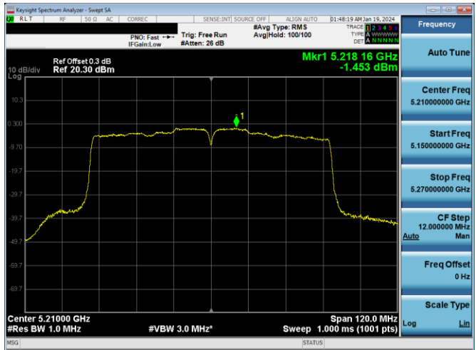
Plot 7-629. PSD CDD PRIMARY Antenna 3c (80MHz BW 802.11ac – Ch. 42, MCS4)
