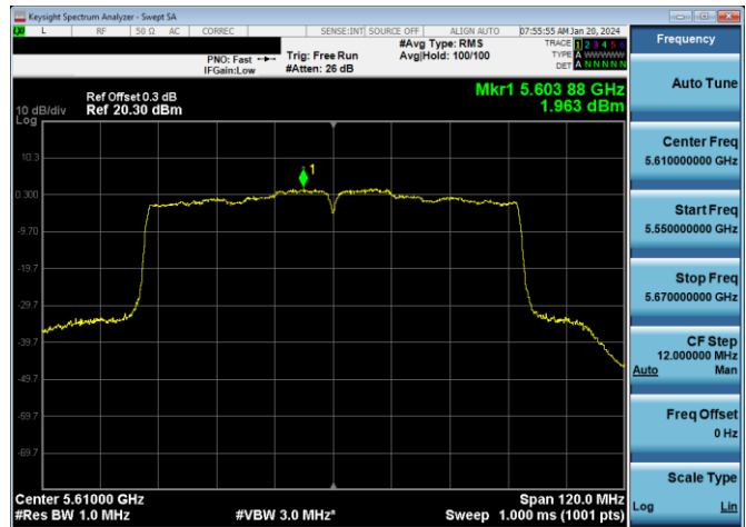
Plot 7-821. PSD CDD DIVERSITY Antenna 1b (80MHz BW 802.11ac – Ch. 122, MCS4)
