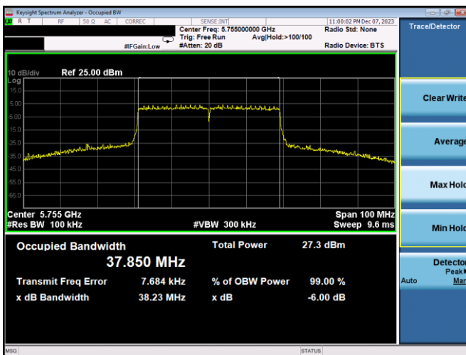
Plot 7-208. 6dB BW & 99% OBW Antenna 3c (40MHz BW 802.11ax(SU) – Ch. 151, MCS4)
