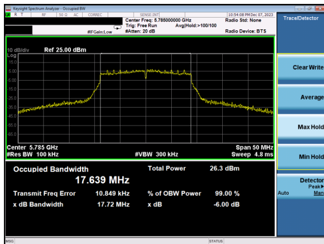
Plot 7-205. 6dB BW & 99% OBW Antenna 3c (20MHz BW 802.11n – Ch. 157, MCS4)
