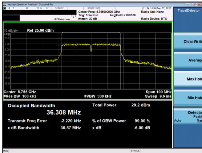
Plot 7-213. 6dB BW & 99% OBW Antenna 3c (40MHz BW 802.11n – Ch. 151, MCS7)
