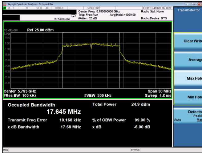
Plot 7-223. 6dB BW & 99% OBW Antenna 3a (20MHz BW 802.11n – Ch. 157, MCS4)
