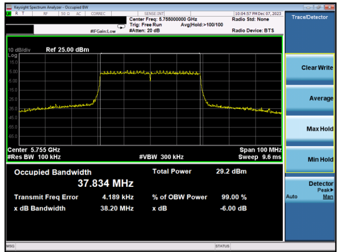
Plot 7-202. 6dB BW & 99% OBW Antenna 3c (40MHz BW 802.11ax(SU) – Ch. 151, MCS2)
