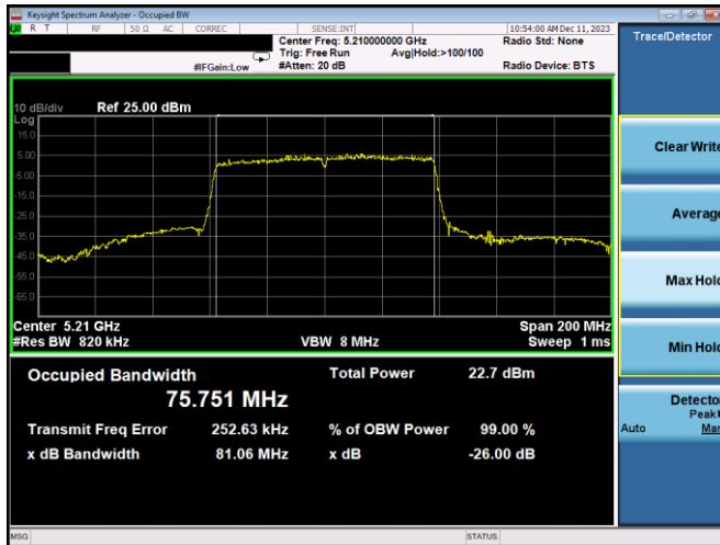
Plot 7-181. 26dB BW & 99% OBW Antenna 1b (80MHz BW 802.11ac – Ch. 42, MCS9)
