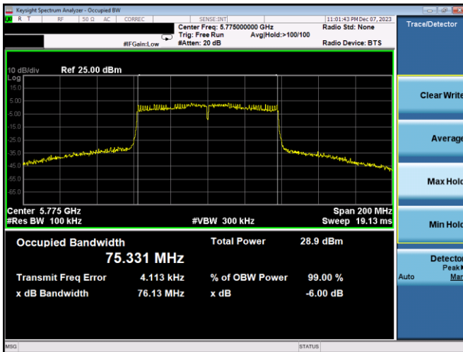
Plot 7-209. 6dB BW & 99% OBW Antenna 3c (80MHz BW 802.11ac – Ch. 155, MCS4)
