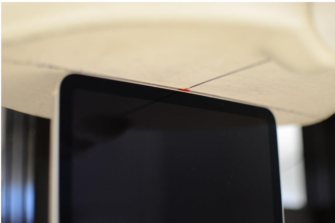
SAR Test Setup Photo 3: Body, Top Edge at 0.0 cm
