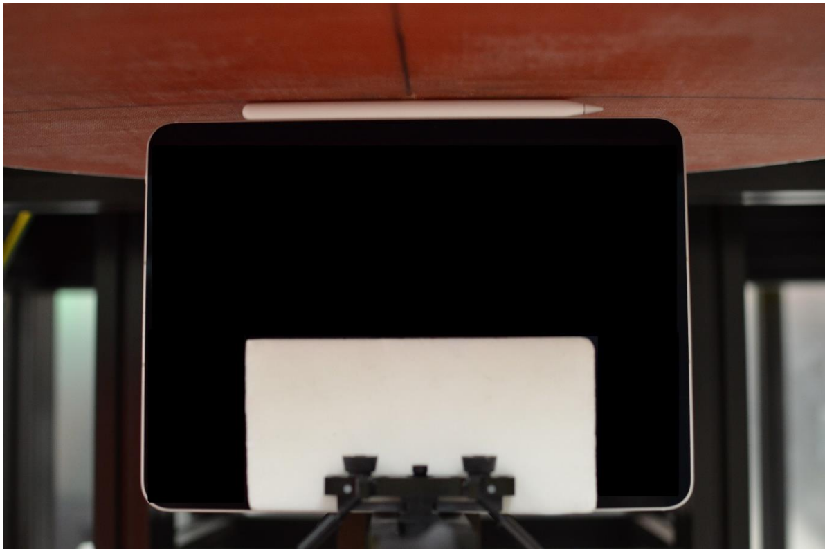
Wireless Power Transfer (wPT) Test Setup Photo 12: Body, Right Edge at 0.0 cm
