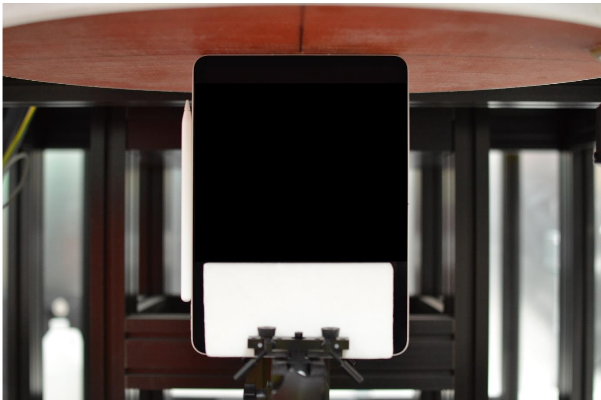
Wireless Power Transfer (wPT) Test Setup Photo 11: Body, Bottom Edge at 0.0 cm
