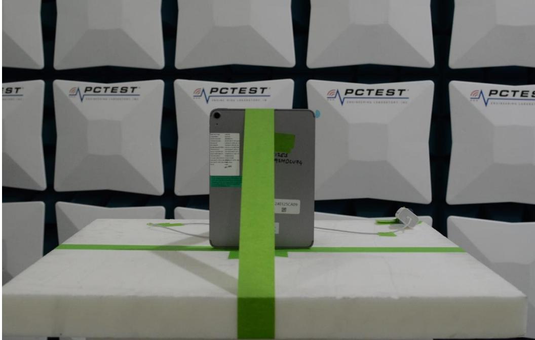
Figure 9: 1-18GHz Test Setup (Front View)
