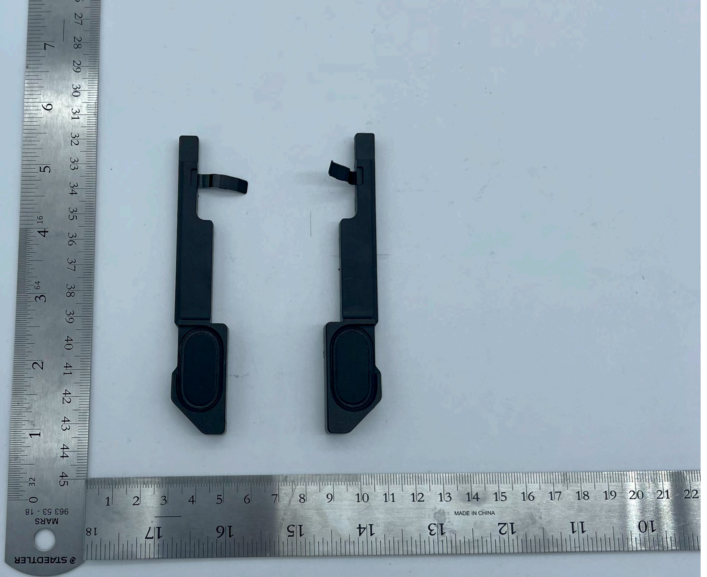
A2918 Left and right speaker structure- Front
