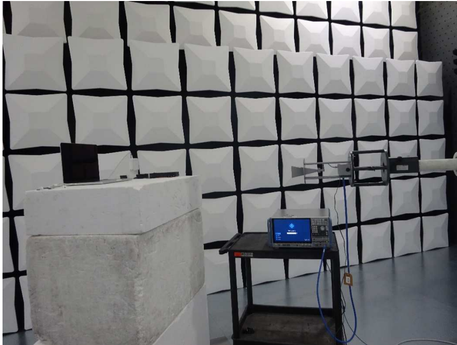
Figure 3 Radiated Disturbance - Above 1 GHz
