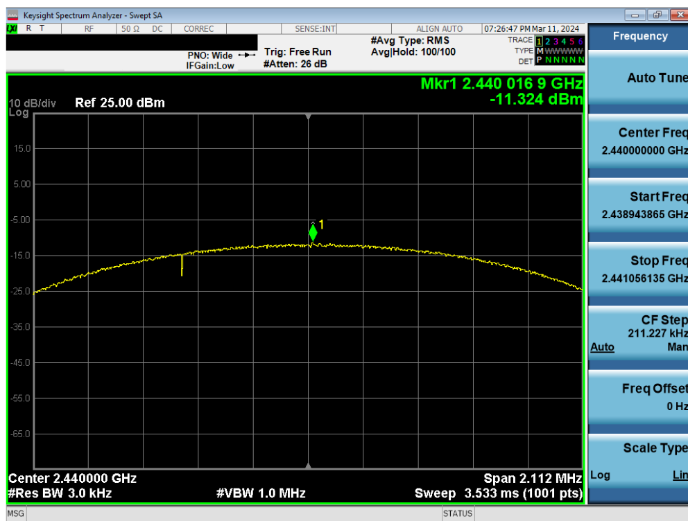
Plot 7-38. Power Spectral Density Plot Antenna WF7 (Bluetooth (LE), 2Mbps, ePA – Ch. 19)
