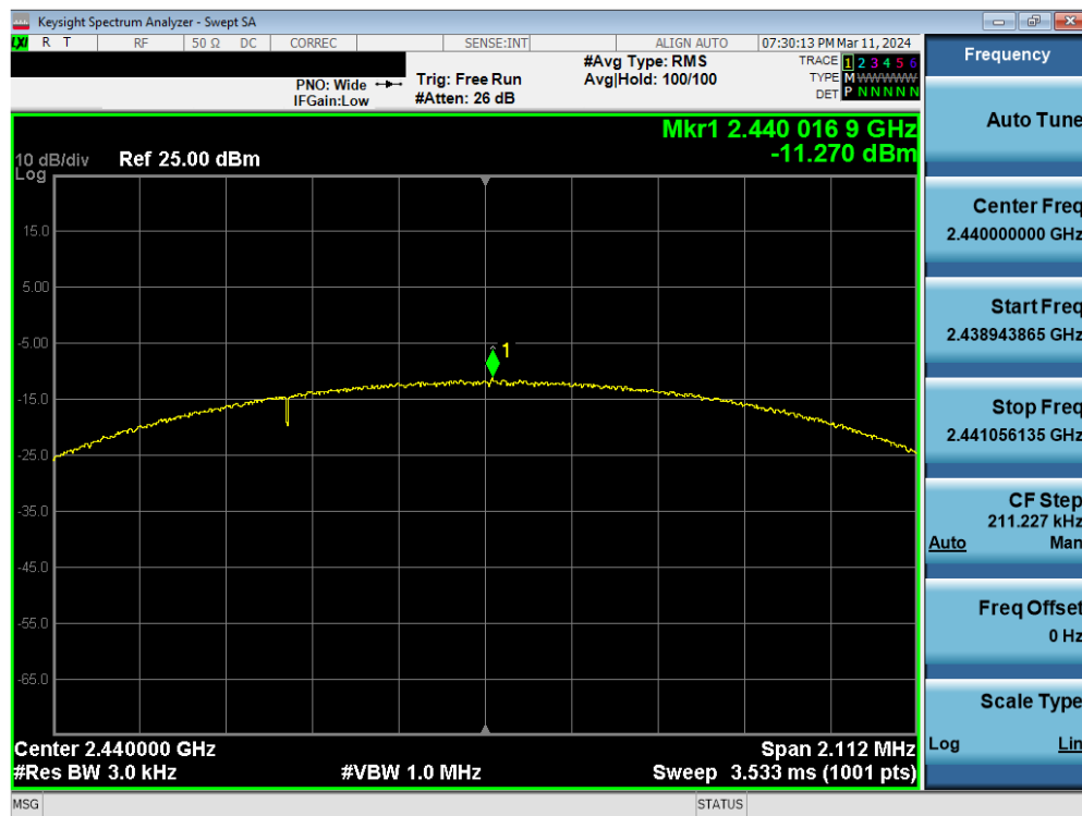
Plot 7-41. Power Spectral Density Plot Antenna WF7 (Bluetooth (LE), 2Mbps, iPA – Ch. 19)
