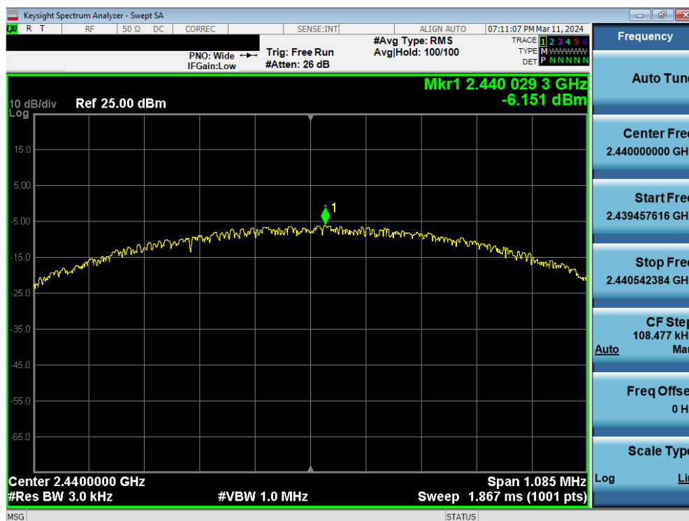
Plot 7-63. Power Spectral Density Plot Antenna WF8 (Bluetooth (LE), 1Mbps, iPA – Ch. 19)
