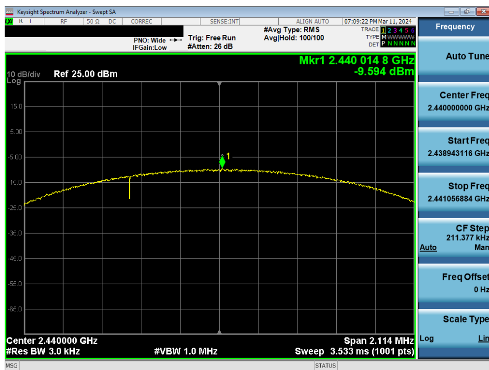
Plot 7-69. Power Spectral Density Plot Antenna WF8 (Bluetooth (LE), 2Mbps, ePA – Ch. 19)
