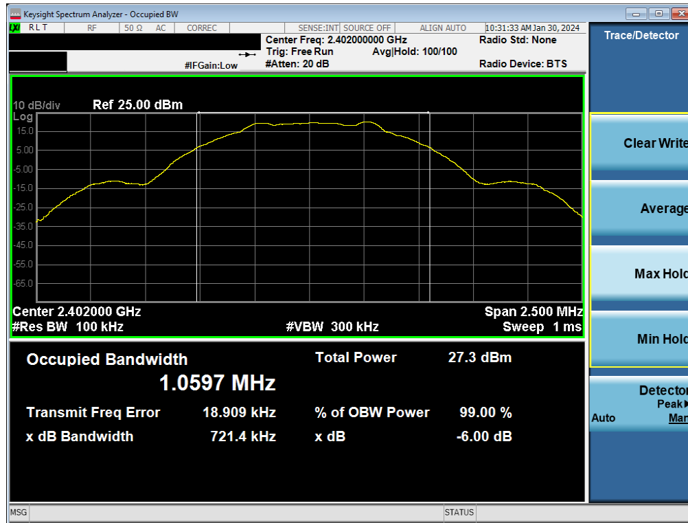
Plot 7-13. 6dB BW & 99% OBW Plot Antenna WF9 (Bluetooth (LE), 1Mbps, ePA – Ch. 0)
