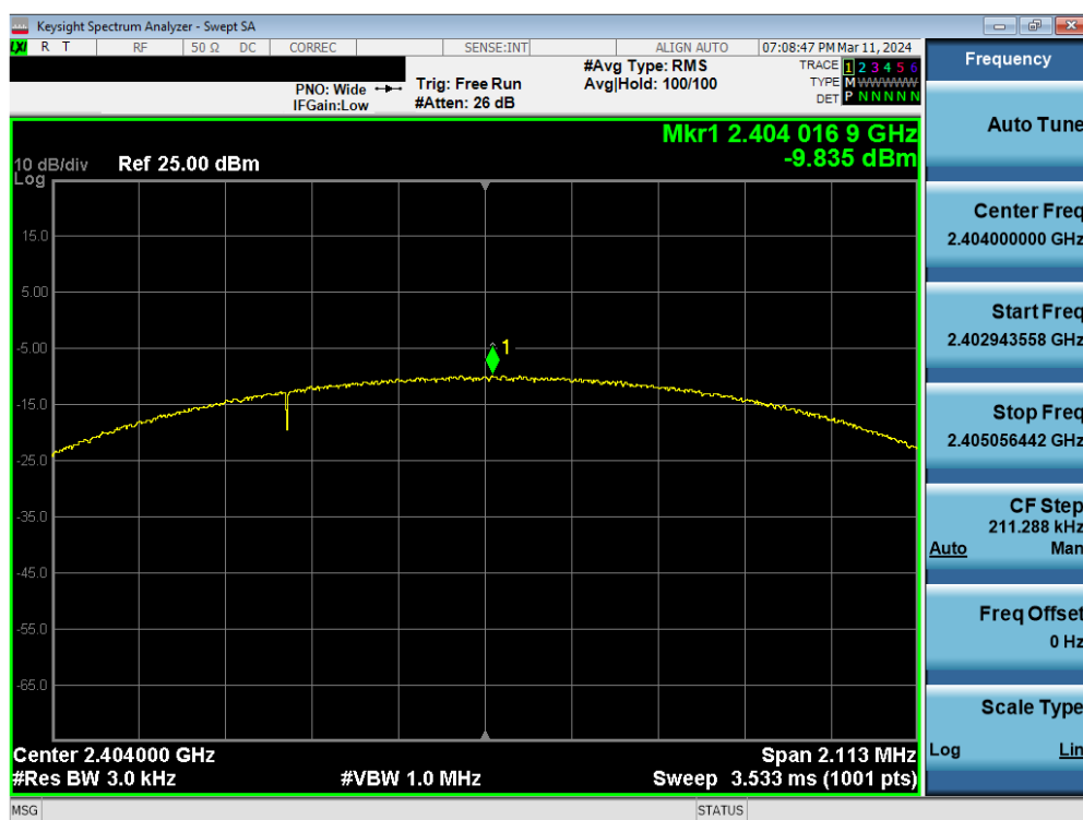
Plot 7-67. Power Spectral Density Plot Antenna WF8 (Bluetooth (LE), 2Mbps, ePA – Ch. 1)
