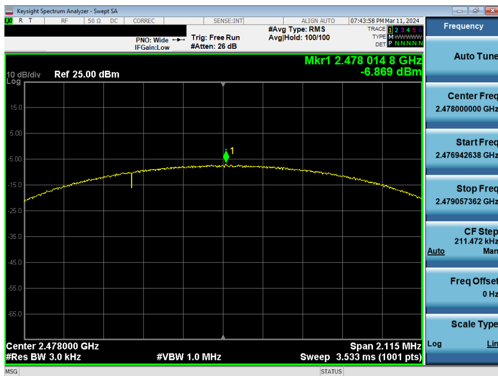
Plot 7-51. Power Spectral Density Plot Antenna WF9 (Bluetooth (LE), 2Mbps, ePA – Ch. 38)
