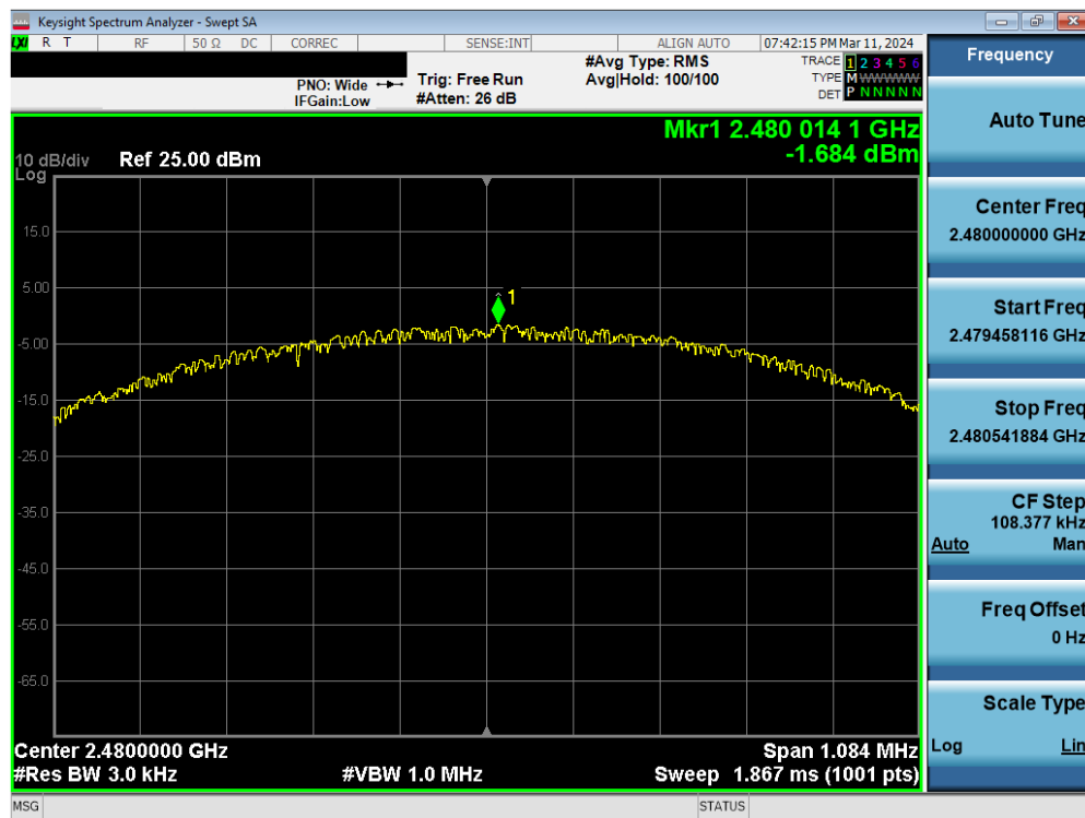
Plot 7-45. Power Spectral Density Plot Antenna WF9 (Bluetooth (LE), 1Mbps, ePA – Ch. 39)
