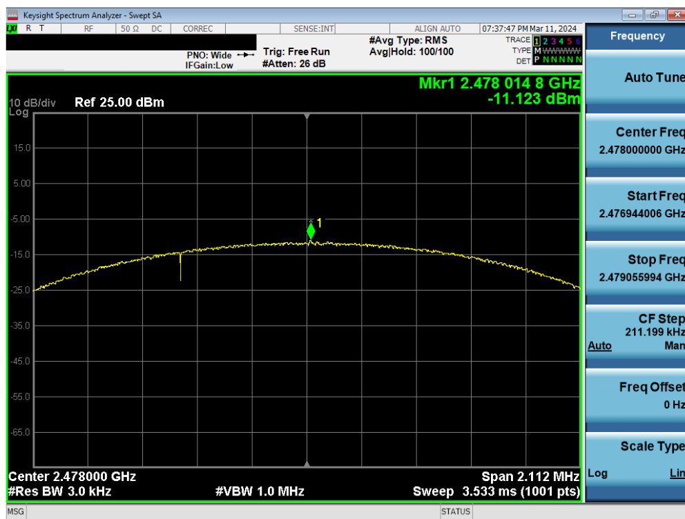
Plot 7-78. Power Spectral Density Plot Antenna WF7 (Bluetooth (LE), 2Mbps, iPA – Ch. 38)
