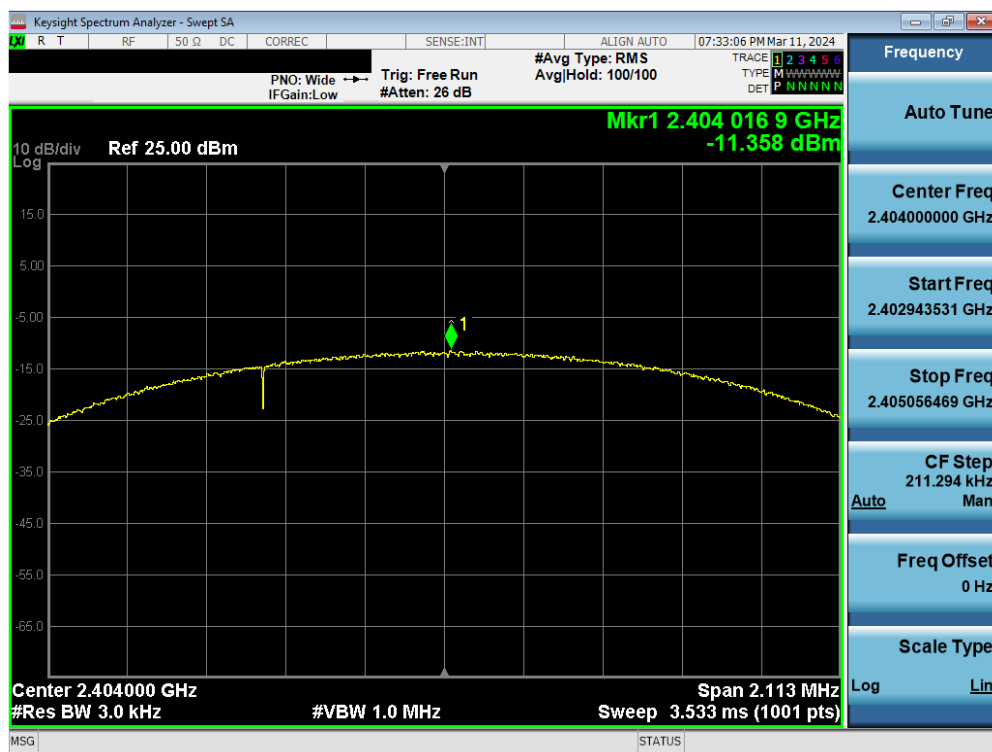
Plot 7-68. Power Spectral Density Plot Antenna WF7 (Bluetooth (LE), 2Mbps, ePA – Ch. 1)
