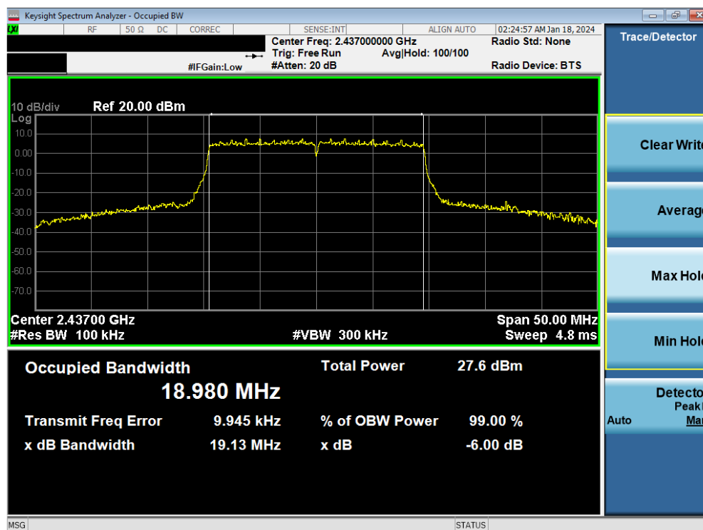
Plot 7-11. 6dB BW & 99% OBW Plot Antenna WF8 (802.11ax OFDMA – RU242 – Ch. 6)
