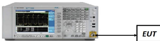
Figure 7-3. Test Instrument & Measurement Setup
