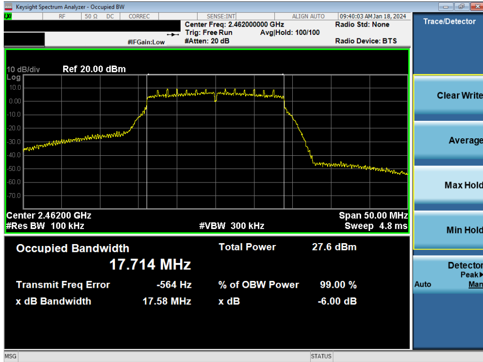
Plot 7-66. 6 dB BW and 99% OBW Plot Antenna WF9 (802.11n (2.4GHz) – Ch. 11) – MCS2
