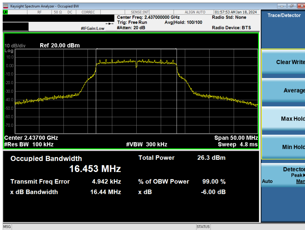
Plot 7-2. 6 dB BW and 99% OBW Plot Antenna WF8 (802.11g – Ch. 6) – 12Mbps
