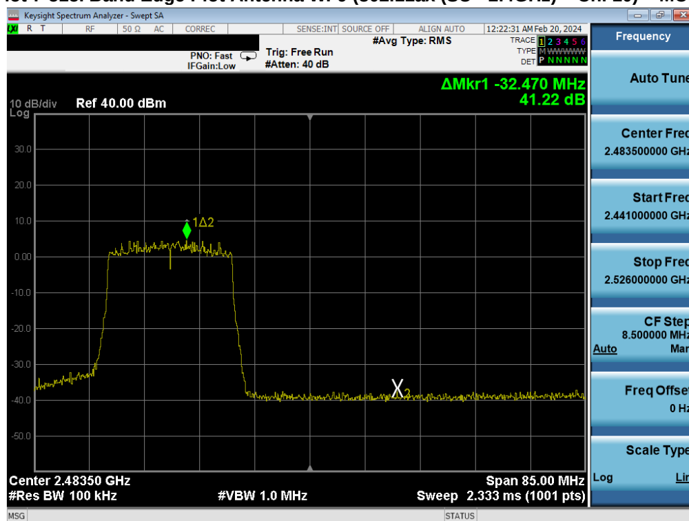
Plot 7-516. Band Edge Plot Antenna WF9 (802.11ax (SU - 2.4GHz) – Ch. 11) – MCS4
