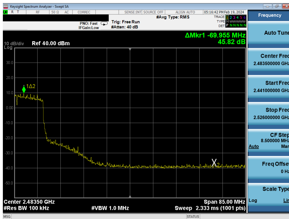
Plot 7-413. Band Edge Plot Antenna WF7 (802.11ax (SU - 2.4GHz) – Ch. 7) – MCS4
