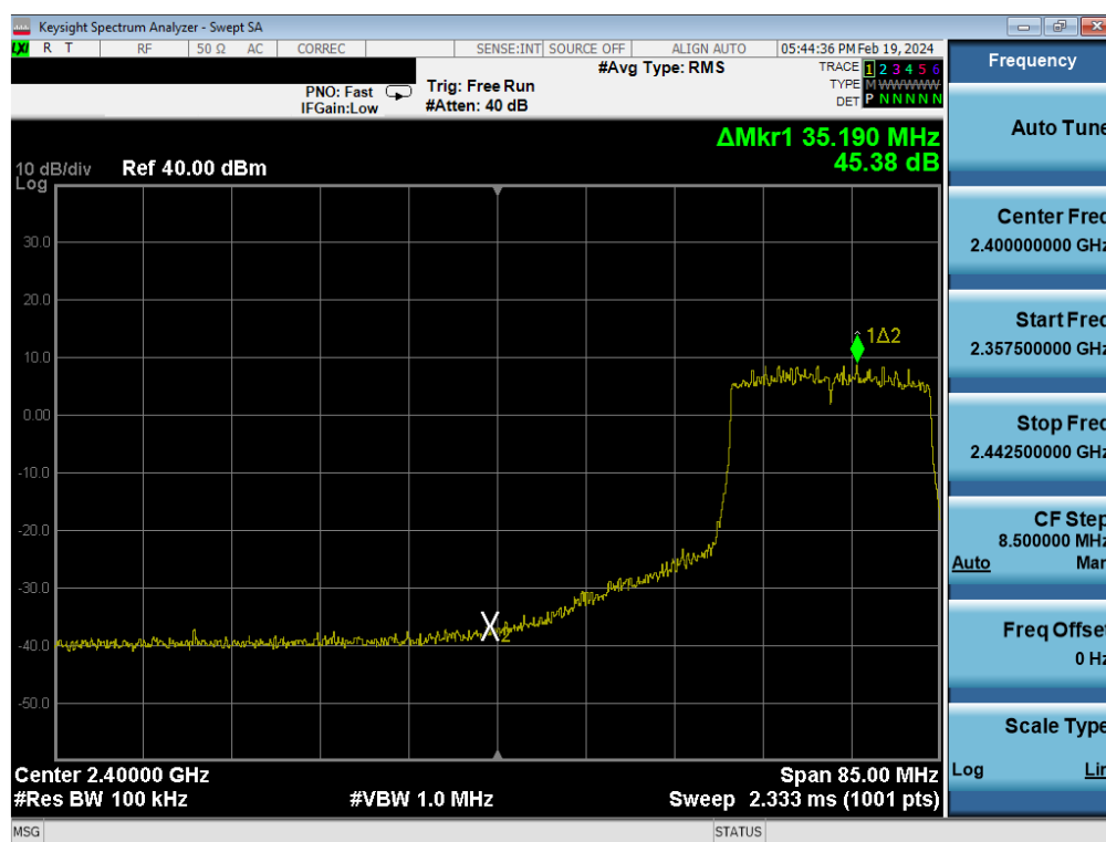
Plot 7-451. Band Edge Plot Antenna WF7 (802.11ax (SU - 2.4GHz) – Ch. 5) – MCS9
