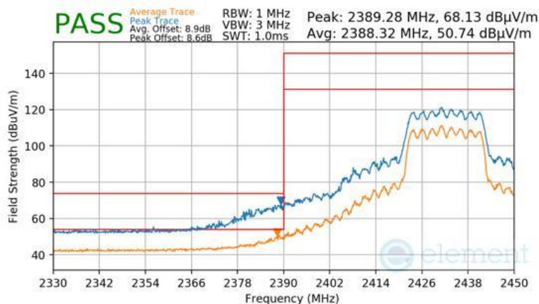
Plot 7-865 Radiated Restricted Lower Band Edge Measurement CDD Primary
