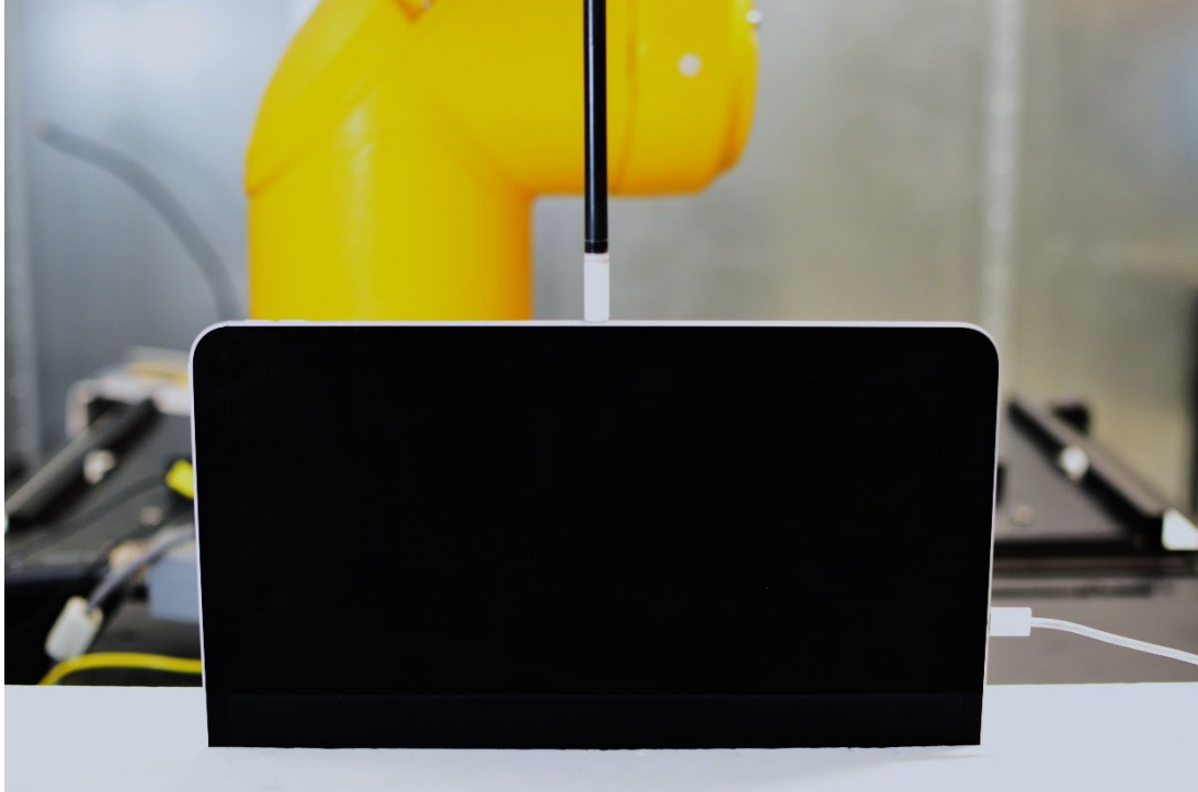
Near Field Power Density Test Setup Photo 18: Right Edge at 2mm – WF7/WF8/WF5B
