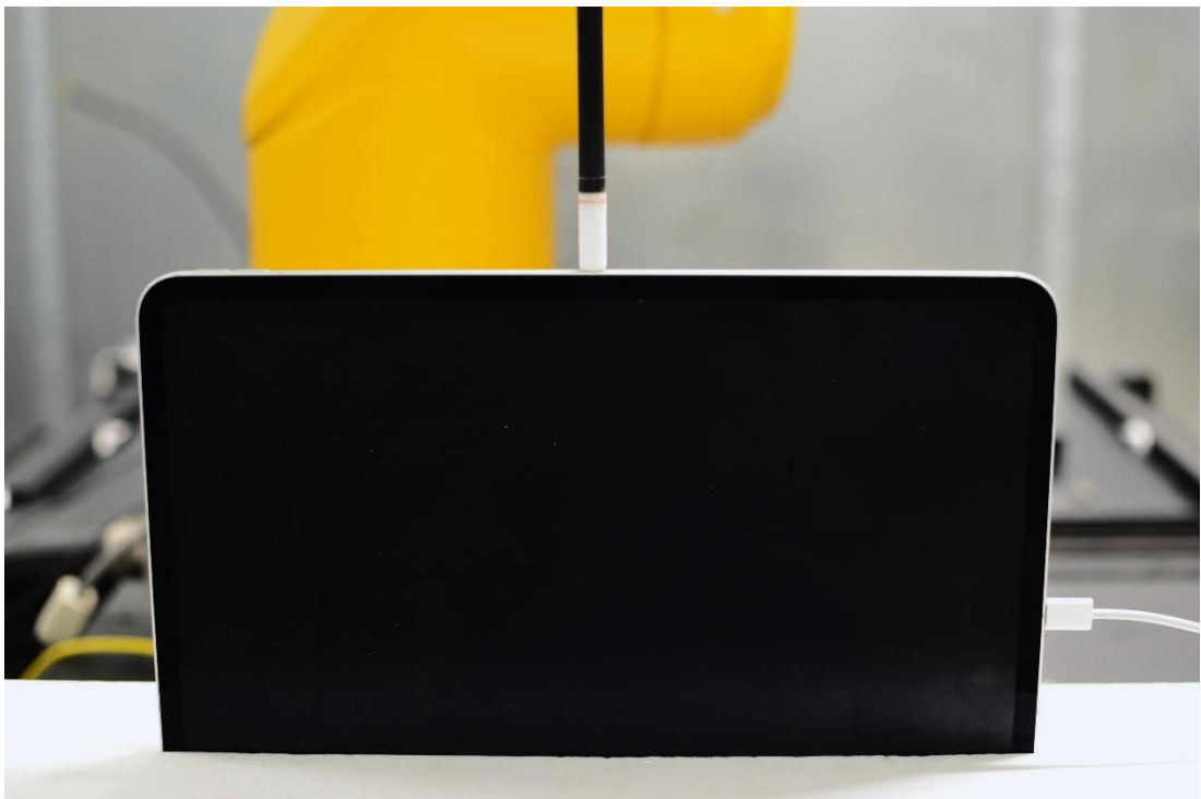
Near Field Power Density Test Setup 12: Right Edge at 2mm – Antenna 2a/4a/WF5B
