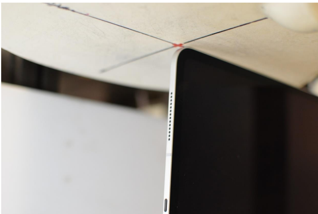
SAR Test Setup Photo 8: Body, Left Edge at 0mm – Antenna 1/2a/2b/WF5B
