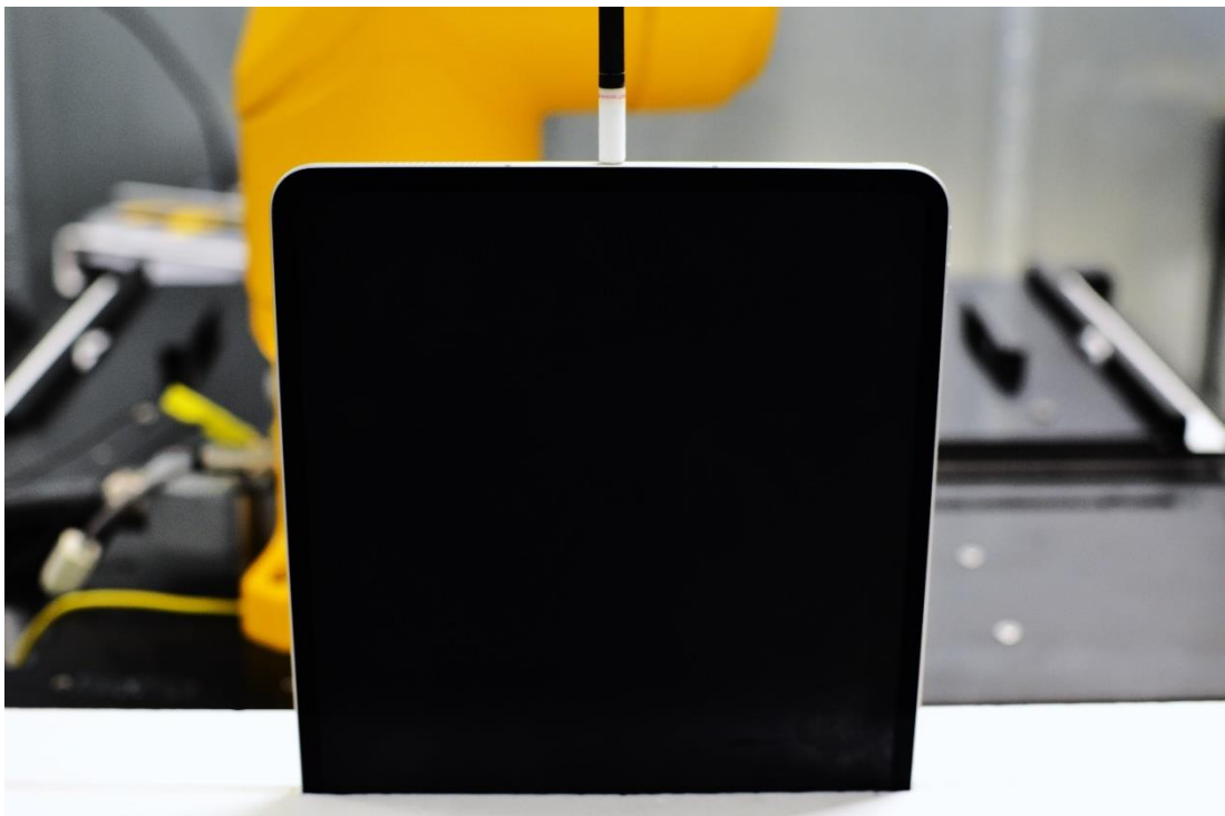
Near Field Power Density Test Setup 10: Top Edge at 2mm – Antenna 2a/4a/WF5B
