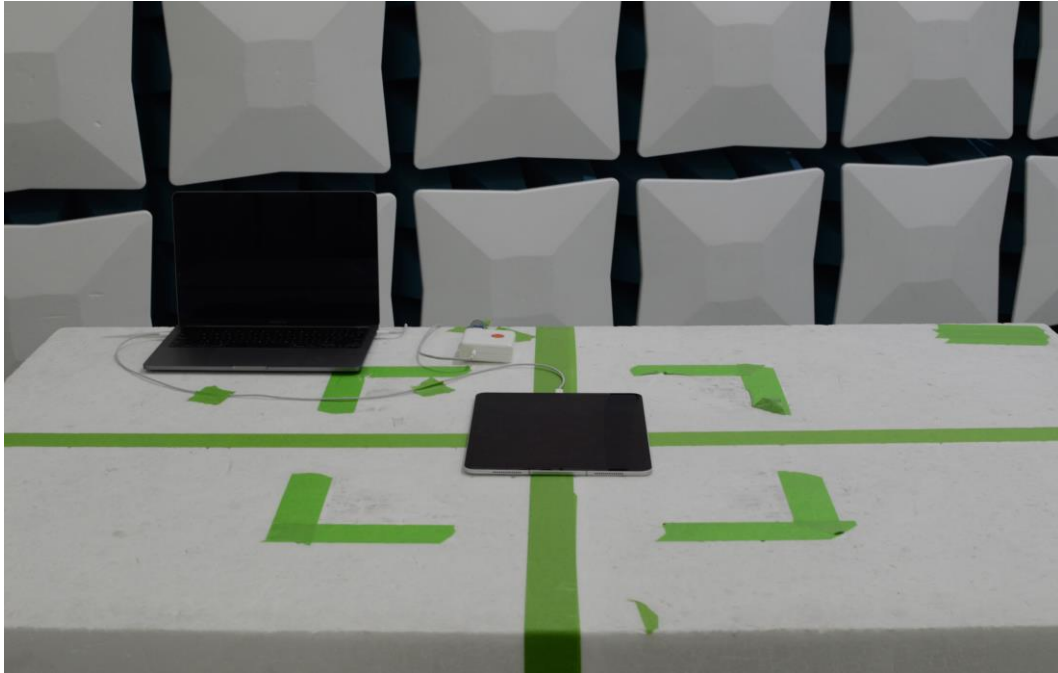
Figure 17: 30MHz-1GHz Test Setup (Front View)
