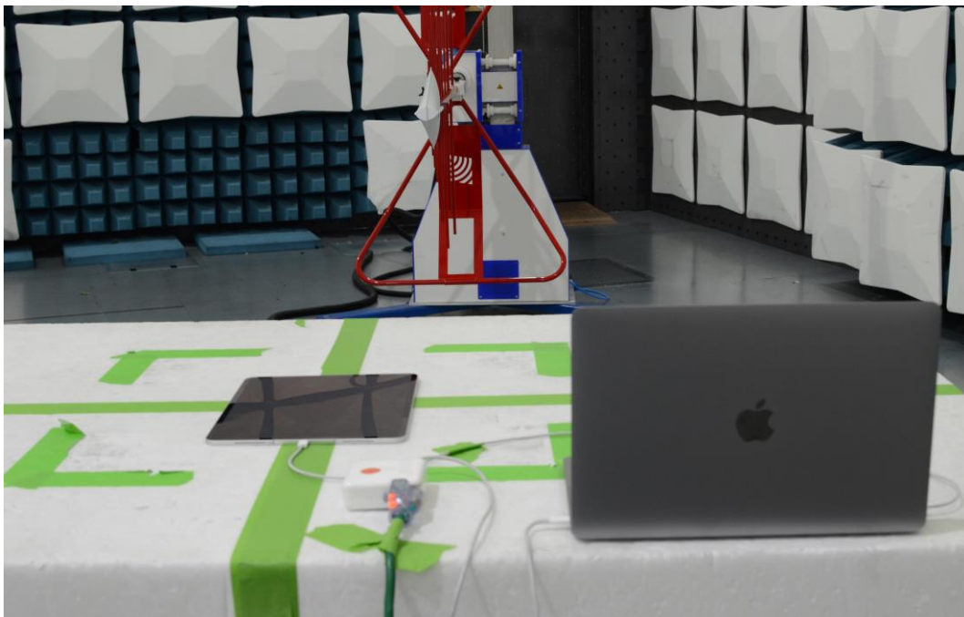
Figure 18: 30MHz-1GHz Test Setup (Rear View)
