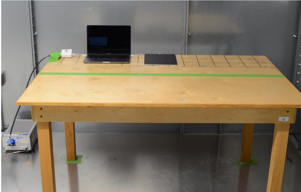
Figure 3: AC Line Conducted Emissions (Front View)
