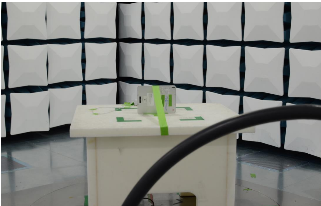
Figure 24: 9kHz-30MHz Test Setup (Front View)
