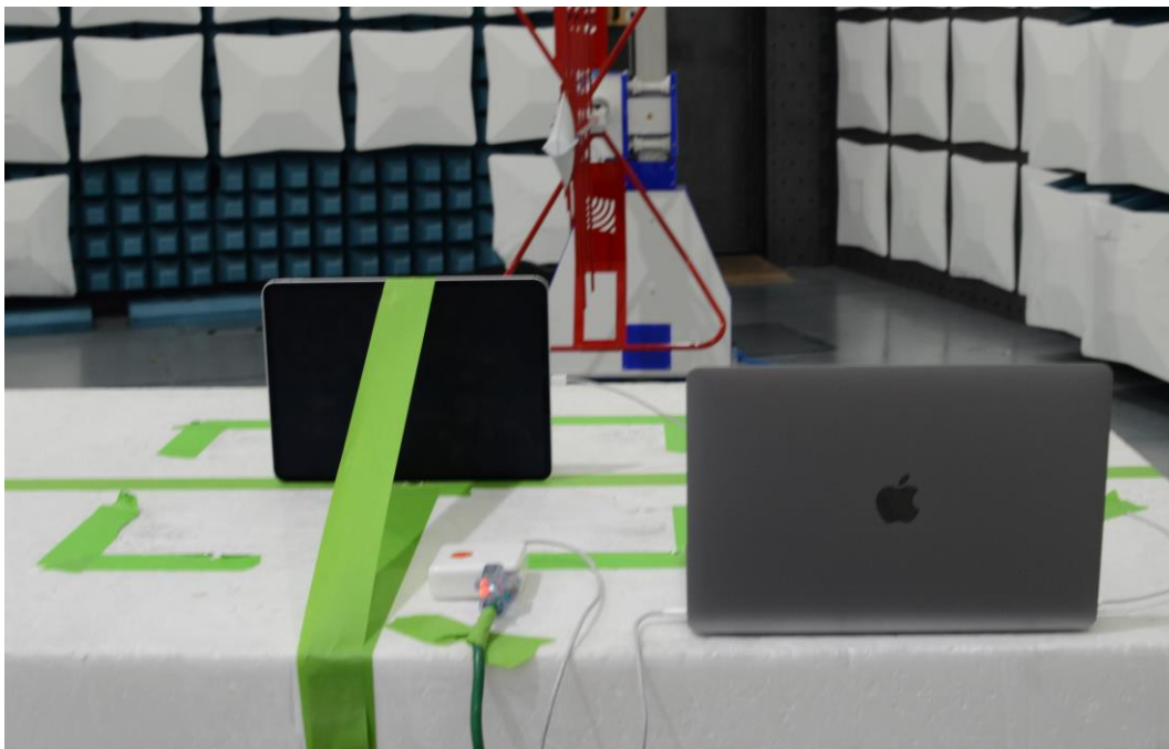
Figure 20: 30MHz-1GHz Test Setup (Rear View)
