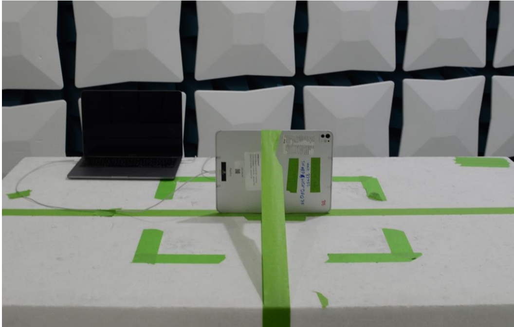
Figure 15: 30MHz-1GHz Test Setup (Front View)
