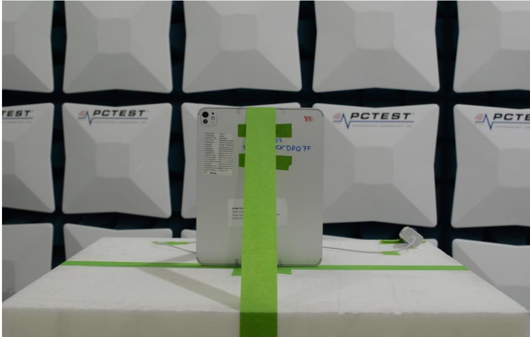
Figure 5: 1-18GHz Test Setup (Front View)
