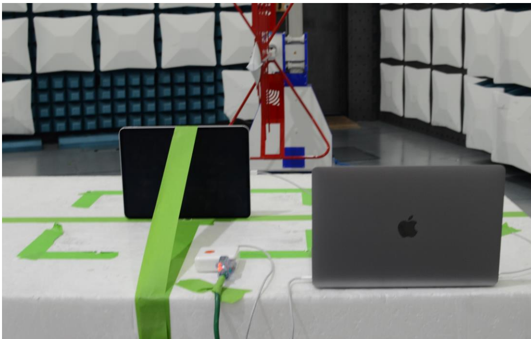
Figure 16: 30MHz-1GHz Test Setup (Rear View)
