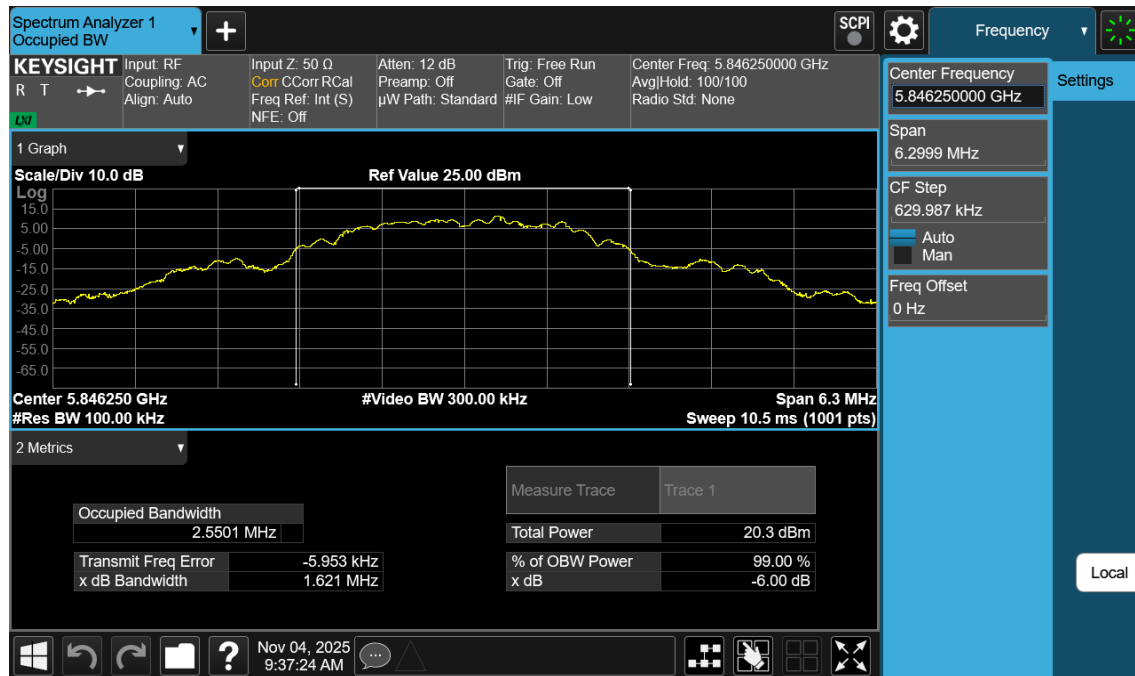
Plot 7-12. 6dB BW OBW (O-QPSK, 5846.25MHz, 250kbps)
