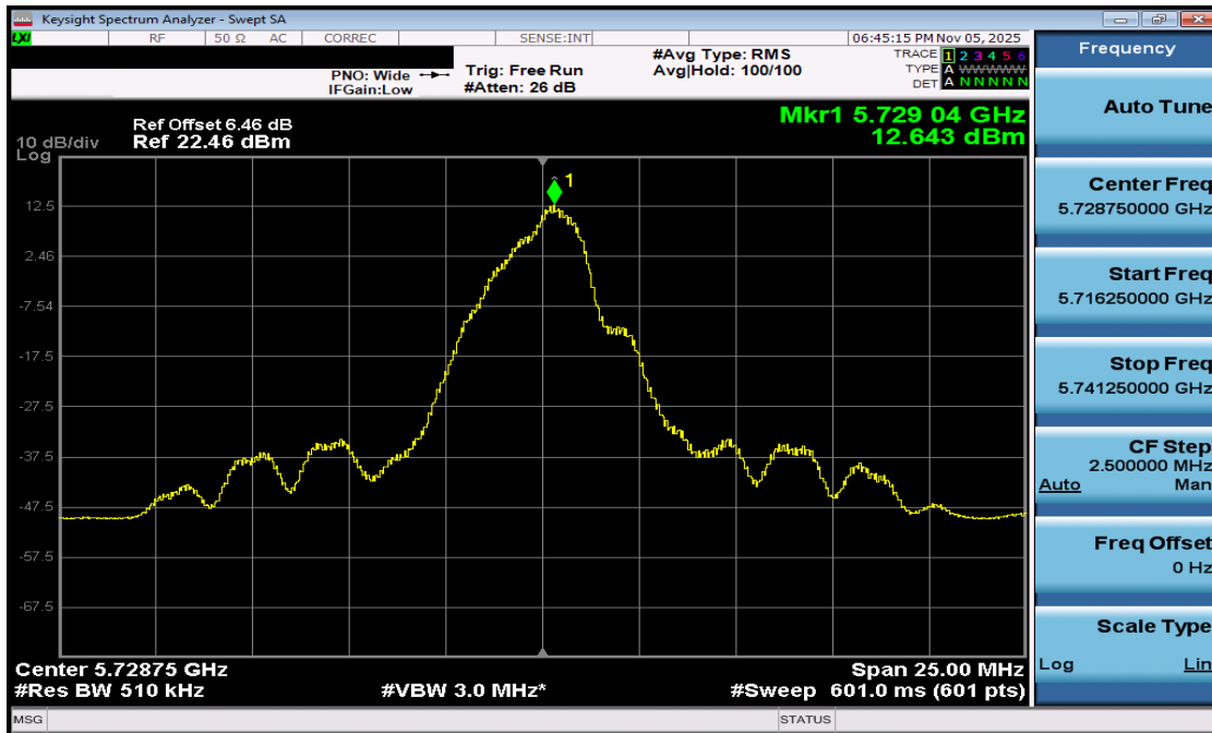
Plot 7-25. PSD (O-QPSK, 5728.75MHz, 1000kbps)
