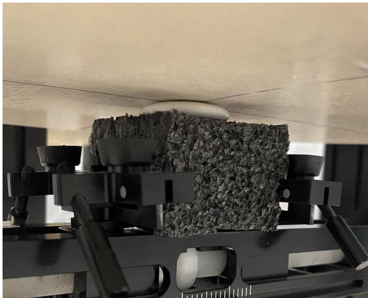
SAR Test Setup Photo 1: Body-worn and Extremity, Front side at 0.0 cm
