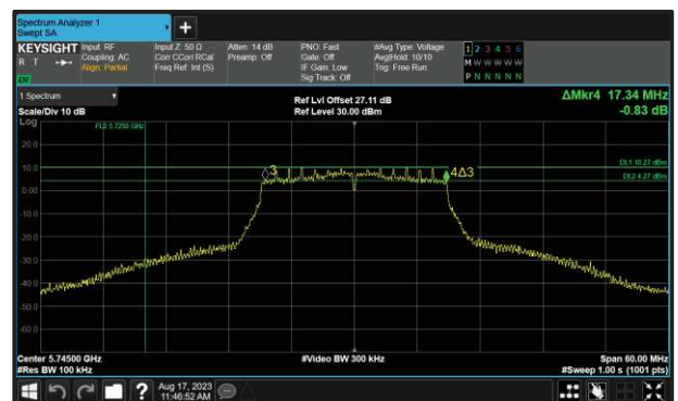
Figure 257 - 802.11n HT20 Maximum 6 dB EBW
