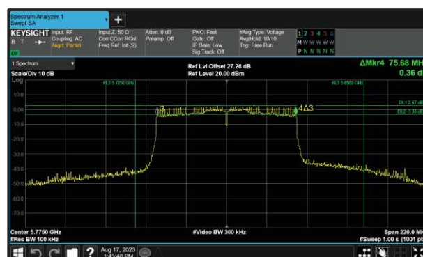
Figure 289 - 802.11ac VHT80 Maximum 6 dB EBW
