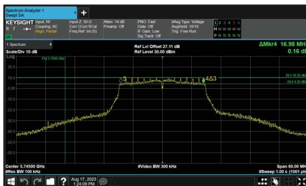
Figure 284 - 802.11n HT20 Minimum 6 dB EBW
