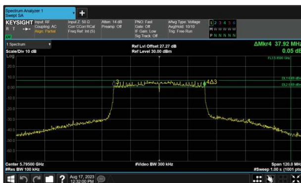
Figure 264 - 802.11ax HE40 SU Minimum 6 dB EBW
