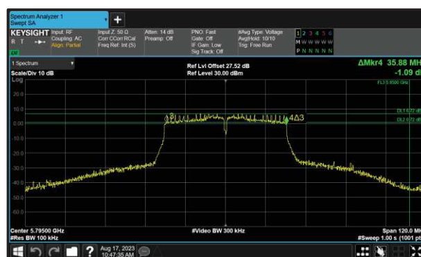
Figure 229 - 802.11n HT40 Maximum 6 dB EBW
