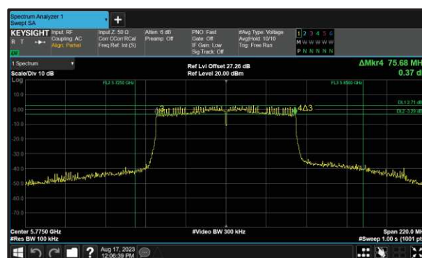
Figure 261 - 802.11ac VHT80 Maximum 6 dB EBW
