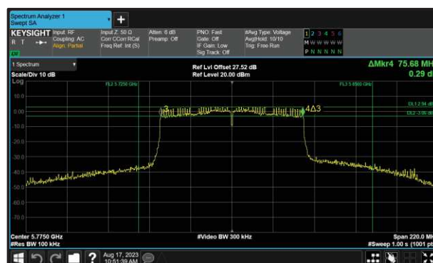
Figure 231 - 802.11ac VHT80 Maximum 6 dB EBW
