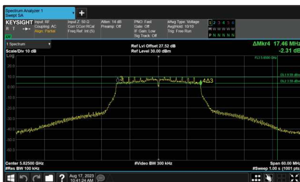
Figure 226 - 802.11n HT20 Minimum 6 dB EBW
