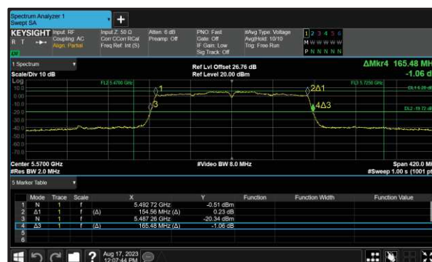
Figure 275 - 802.11ac VHT160 Maximum 99% OBW
