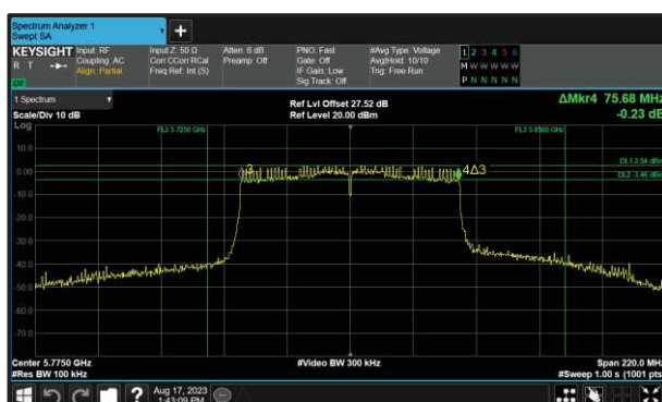
Figure 288 - 802.11ac VHT80 Minimum 6 dB EBW
