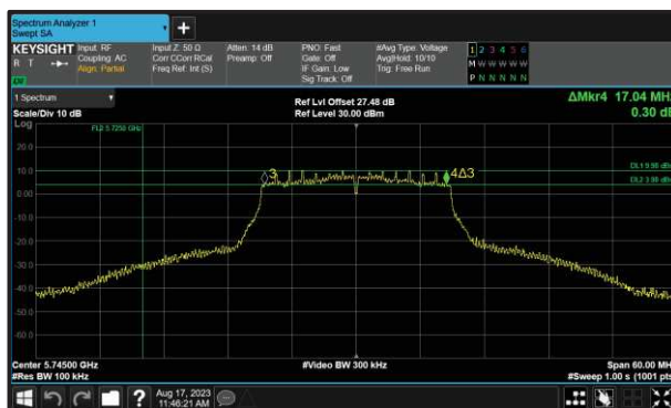
Figure 256 - 802.11n HT20 Minimum 6 dB EBW
