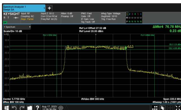
Figure 266 - 802.11ax HE80 SU Minimum 6 dB EBW
