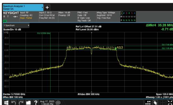
Figure 286 - 802.11n HT40 Minimum 6 dB EBW
