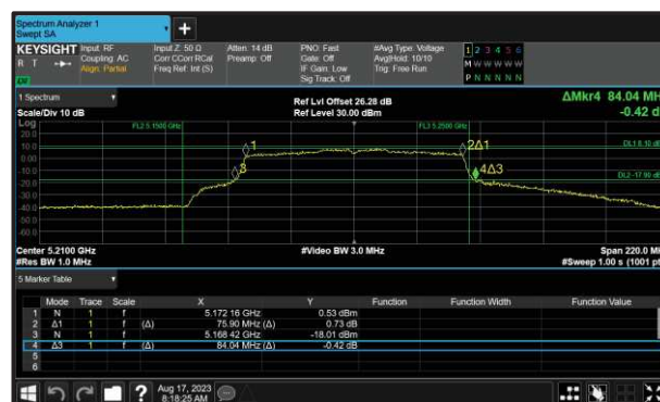
Figure 273 - 802.11ac VHT80 Maximum 99% OBW
