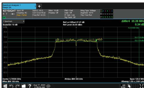
Figure 258 - 802.11n HT40 Minimum 6 dB EBW
