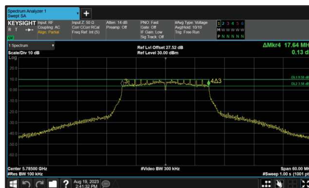
Figure 227 - 802.11n HT20 Maximum 6 dB EBW
