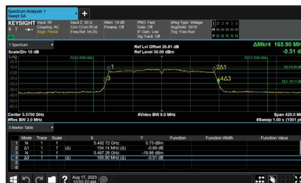
Figure 247 - 802.11ac VHT160 Maximum 99% OBW
