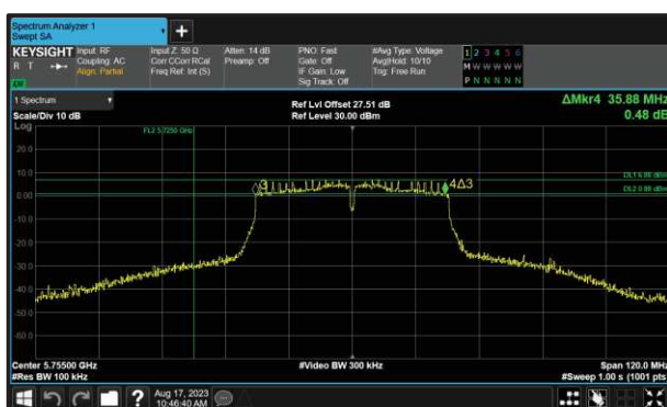
Figure 228 - 802.11n HT40 Minimum 6 dB EBW
