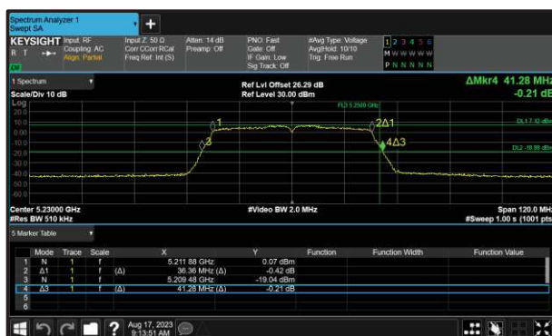
Figure 242 - 802.11n HT40 Minimum 99% OBW
