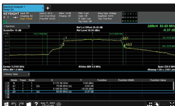
Figure 244 - 802.11ac VHT80 Minimum 99% OBW
