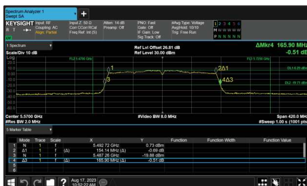
Figure 246 - 802.11ac VHT160 Minimum 99% OBW
