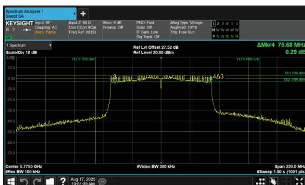
Figure 230 - 802.11ac VHT80 Minimum 6 dB EBW
