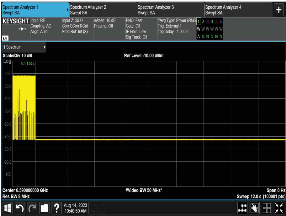
Figure 296 - U-NII-7, Minimum Bandwidth (AWGN Mid)
