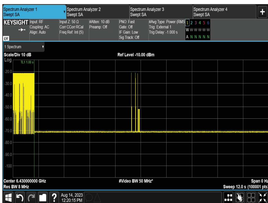
Figure 291 - U-NII-6, Minimum Bandwidth (AWGN Low)
