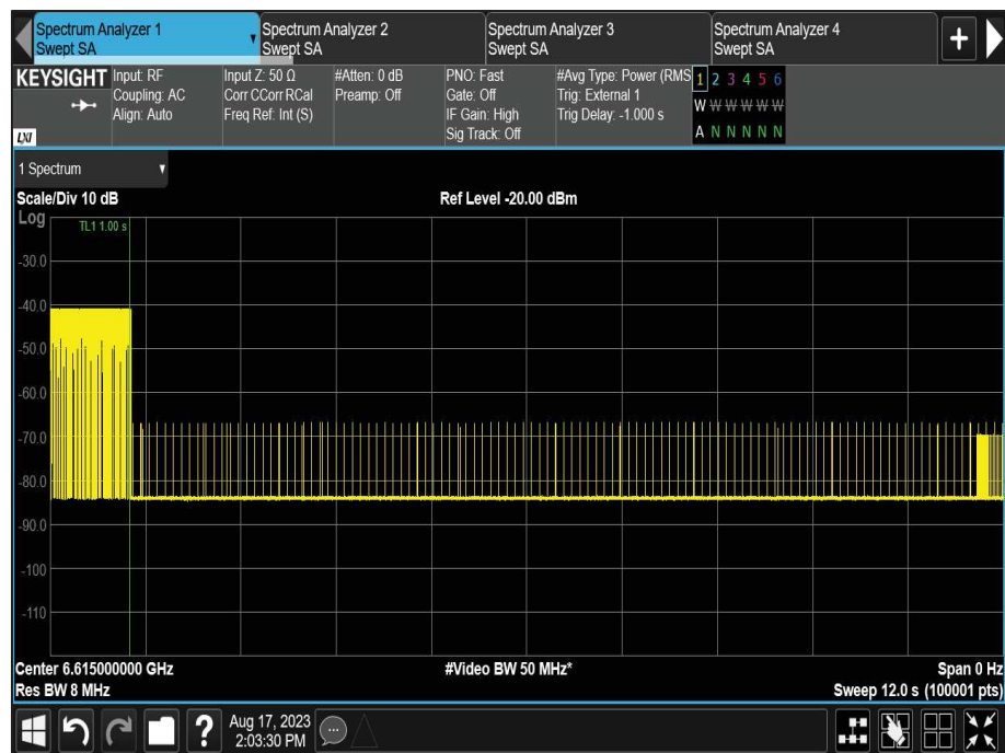
Figure 297 - U-NII-7, Minimum Bandwidth (AWGN High)
