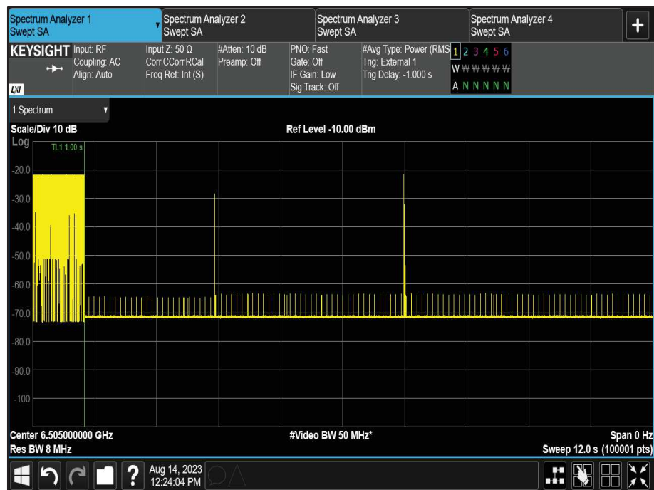
Figure 292 - U-NII-6, Minimum Bandwidth (AWGN Mid)
