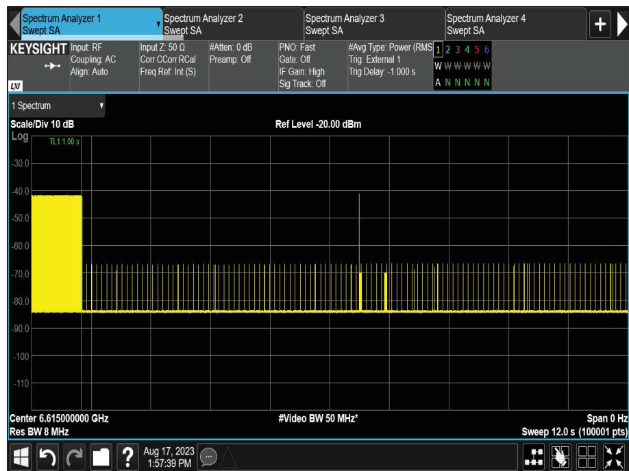
Figure 295 - U-NII-7, Minimum Bandwidth (AWGN Low)
