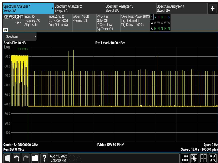
Figure 288 - U-NII-5, Minimum Bandwidth (AWGN Mid)
