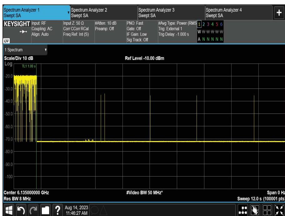
Figure 287 - U-NII-5, Minimum Bandwidth (AWGN Low)
