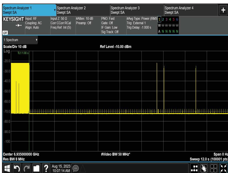
Figure 301 - U-NII-8, Minimum Bandwidth (AWGN High)
