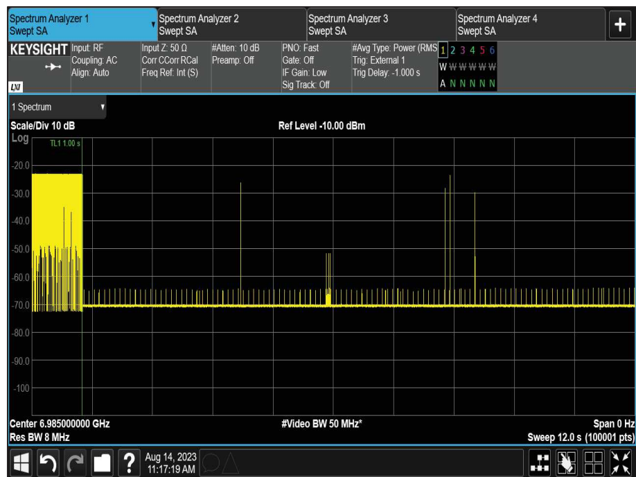
Figure 300 - U-NII-8, Minimum Bandwidth (AWGN Mid)
