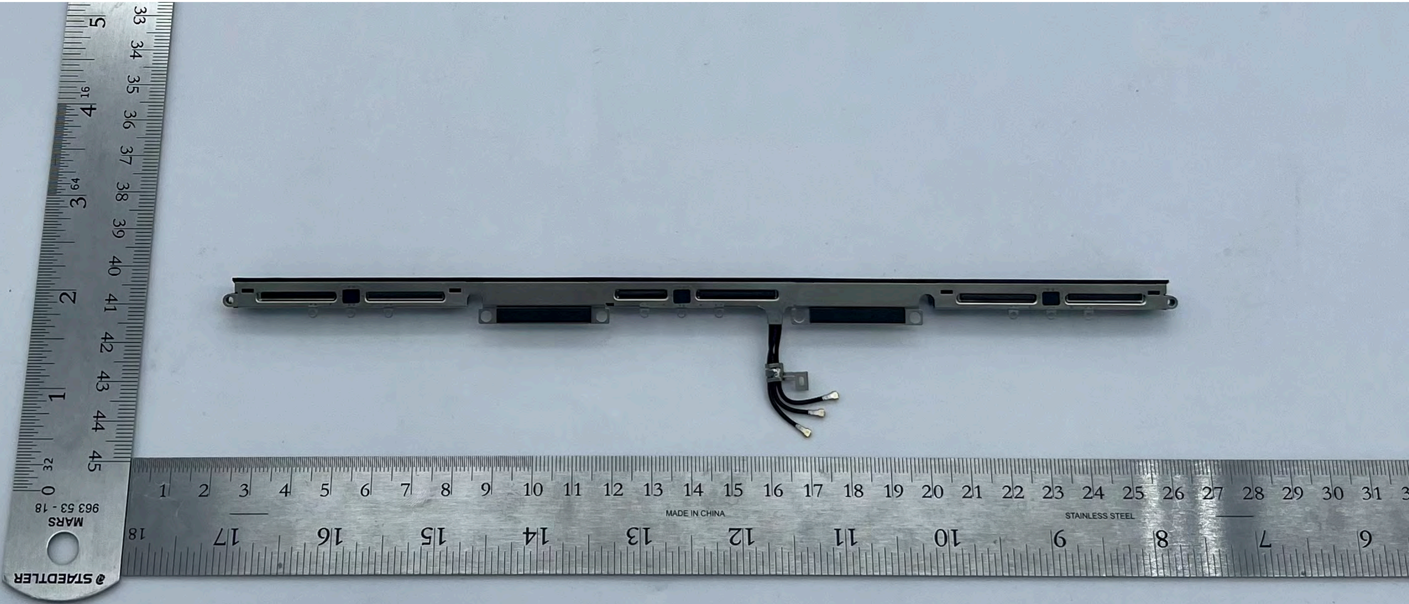
A2992 WF1/BT, WF2/BT, WF3 (BT) antenna structure and feed - Front
