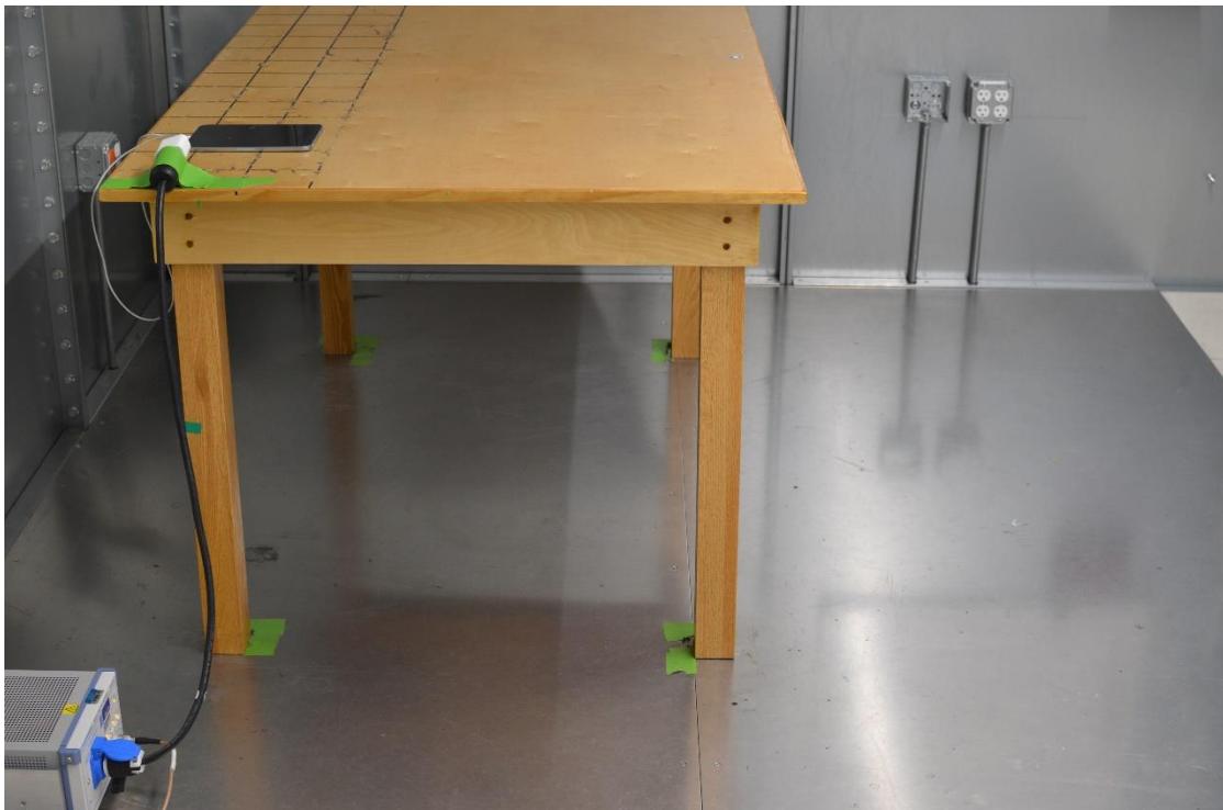
Figure 2: AC Line Conducted Emissions (Side View)
