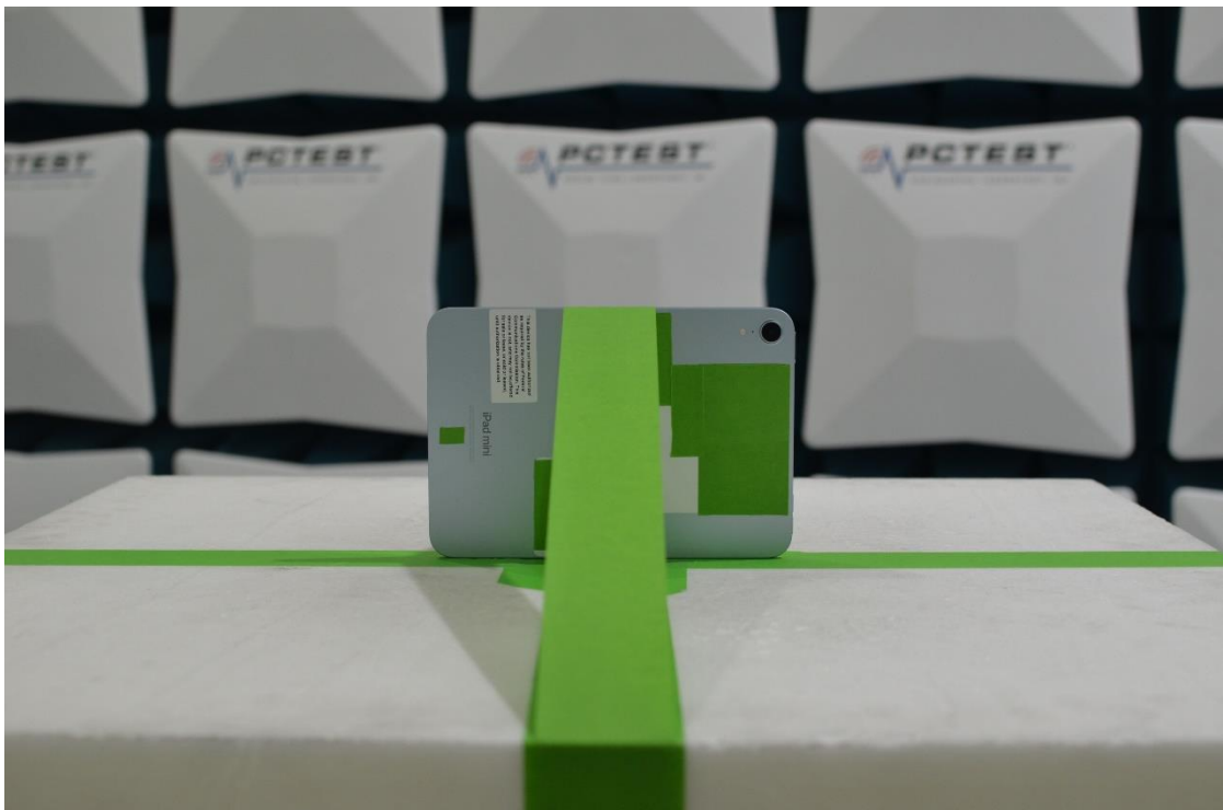
Figure 7: 1-18GHz Test Setup (Front View)
