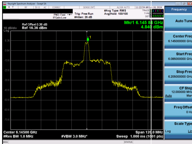
Plot 7-493. SP Power Spectral Density Plot CDD Antenna 5T (80MHz 802.11ax RU26 (UNII Band 5) – Ch. 39)
