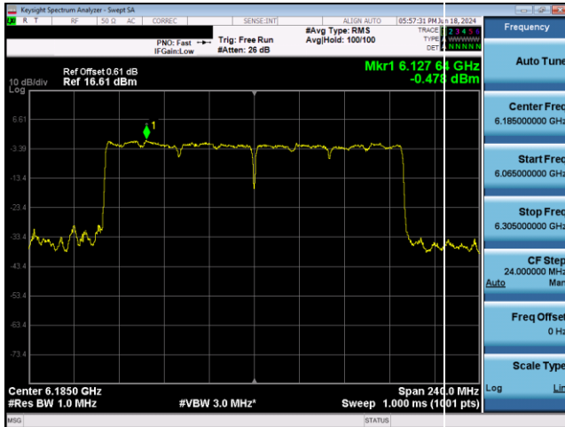
Plot 7-506. SP Power Spectral Density Plot CDD Antenna 3b (160MHz 802.11ax RU996x2 (UNII Band 5) – Ch. 47)
