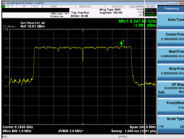
Plot 7-505. SP Power Spectral Density Plot CDD Antenna 5T (160MHz 802.11ax RU996x2 (UNII Band 5) – Ch. 47)
