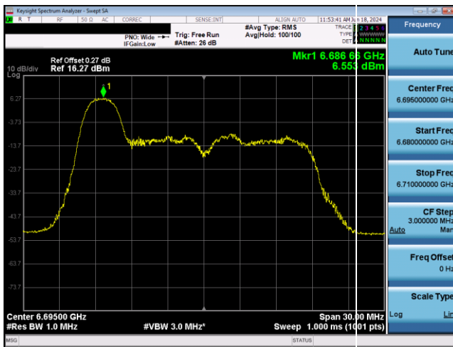
Plot 7-507. SP Power Spectral Density Plot CDD Antenna 5T (20MHz 802.11ax RU26 (UNII Band 7) – Ch. 149)
