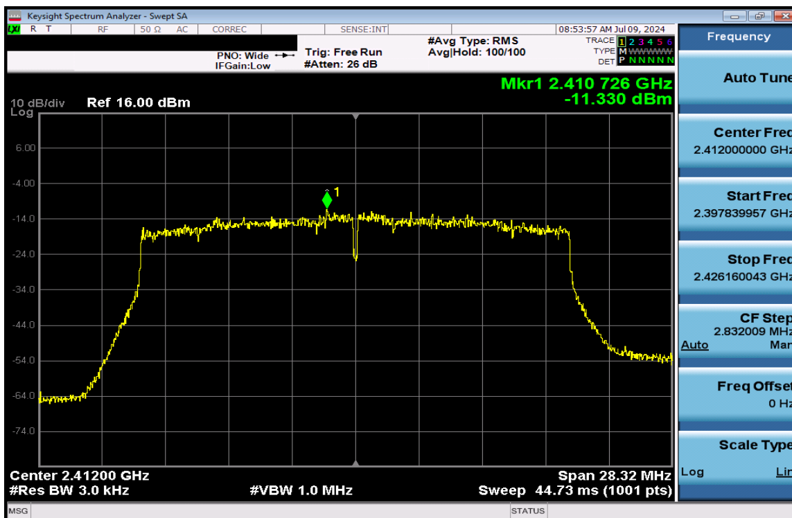
Plot 7-152. Power Spectral Density Plot CDD Antenna 1a (802.11ax (SU - 2.4GHz) – Ch. 1) – MCS4
