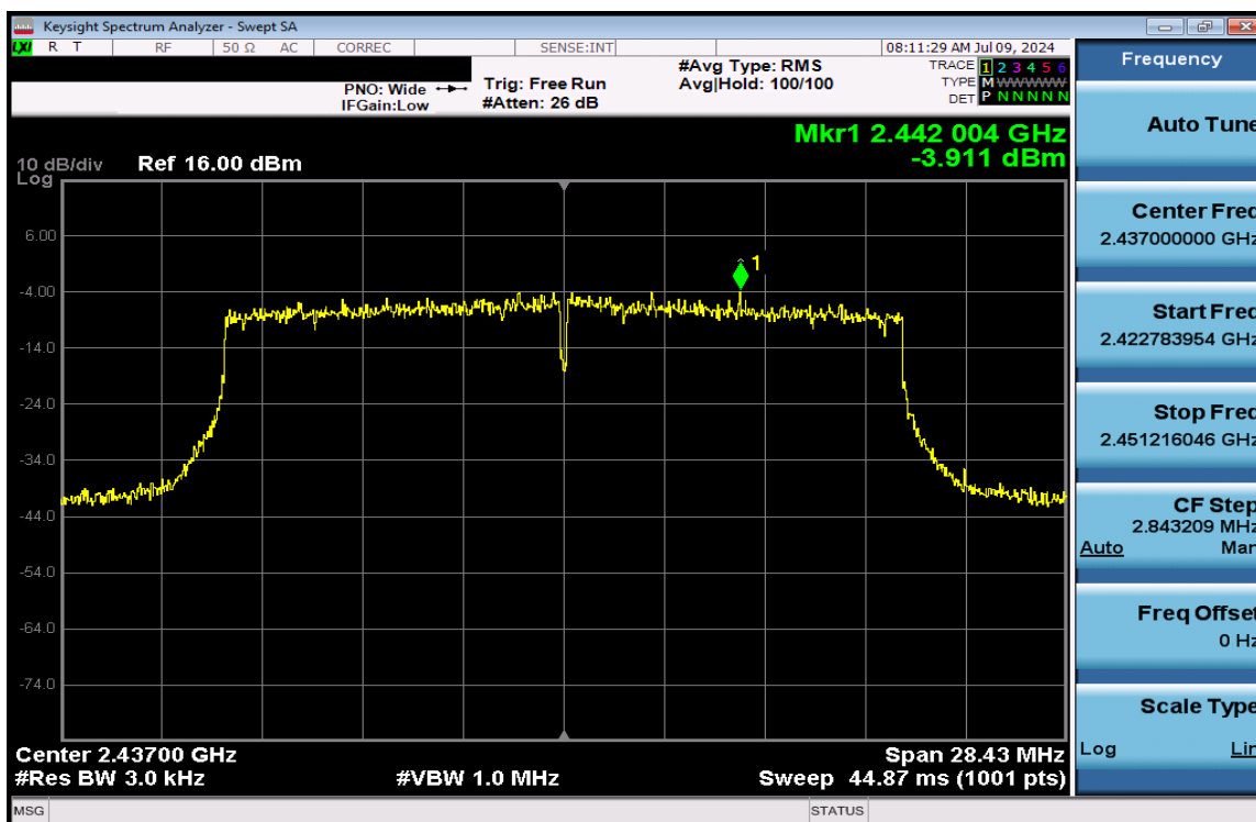
Plot 7-153. Power Spectral Density Plot CDD Antenna 3a (802.11ax (SU - 2.4GHz) – Ch. 6) – MCS4
