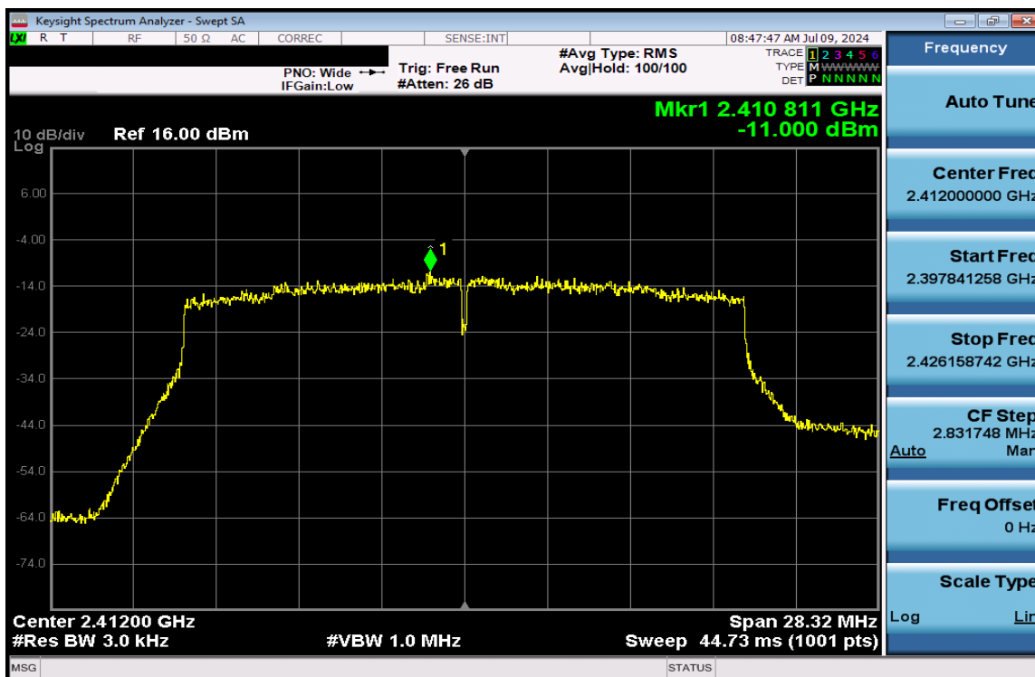
Plot 7-134. Power Spectral Density Plot CDD Antenna 1a (802.11ax (SU - 2.4GHz) – Ch. 1) – MCS2
