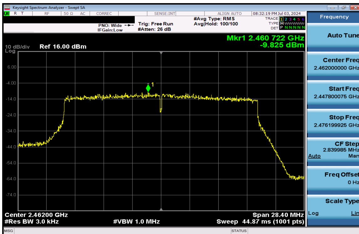
Plot 7-99. Power Spectral Density Plot Antenna 1a (802.11ax (SU - 2.4GHz) – Ch. 11) – MCS2
