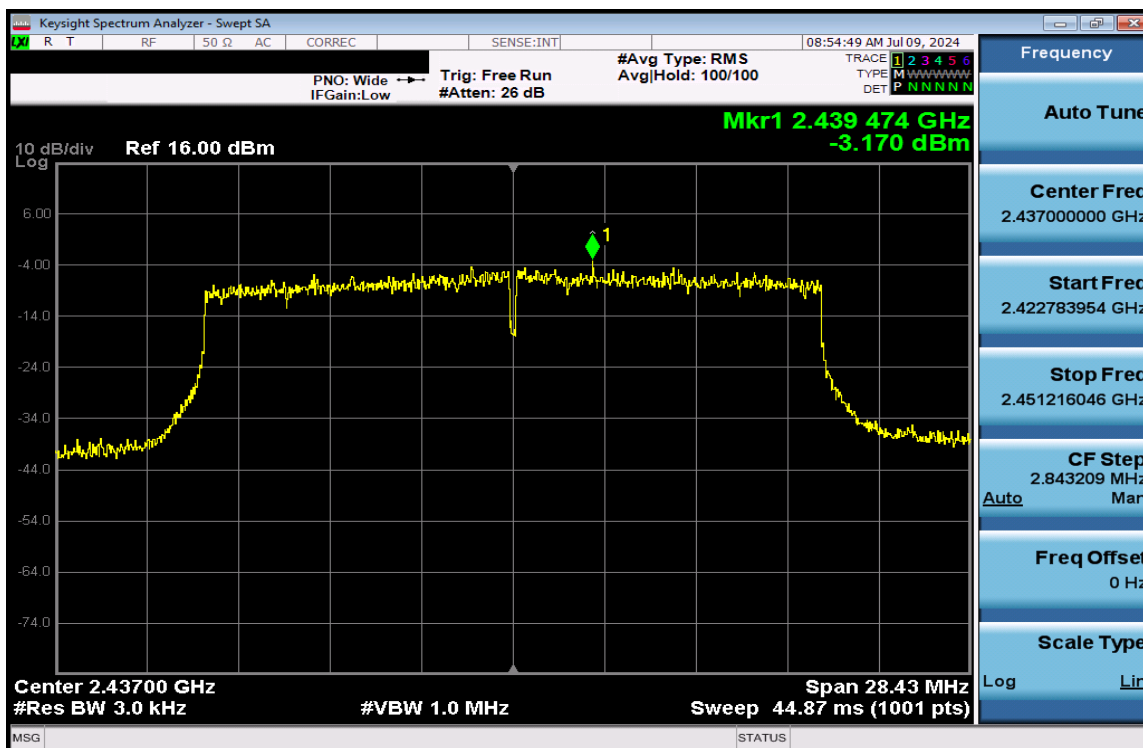
Plot 7-154. Power Spectral Density Plot CDD Antenna 1a (802.11ax (SU - 2.4GHz) – Ch. 6) – MCS4
