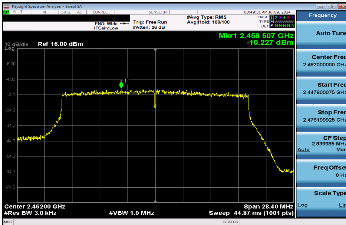
Plot 7-138. Power Spectral Density Plot CDD Antenna 1a (802.11ax (SU - 2.4GHz) – Ch. 11) – MCS2
