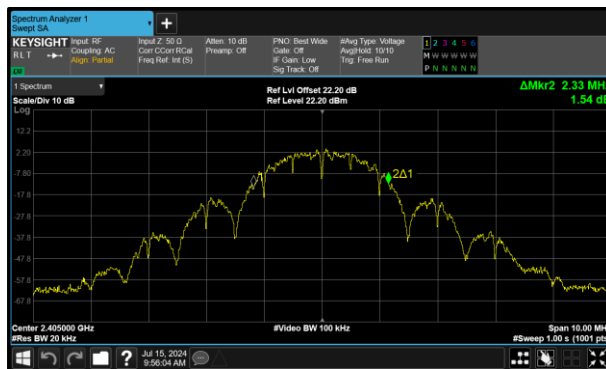
Figure 35 - Core 2 (C) 2405 MHz (CH11) 99% Bandwidth
