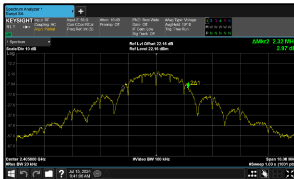
Figure 23 - Core 1 (B) 2405 MHz (CH11) 99% Bandwidth
