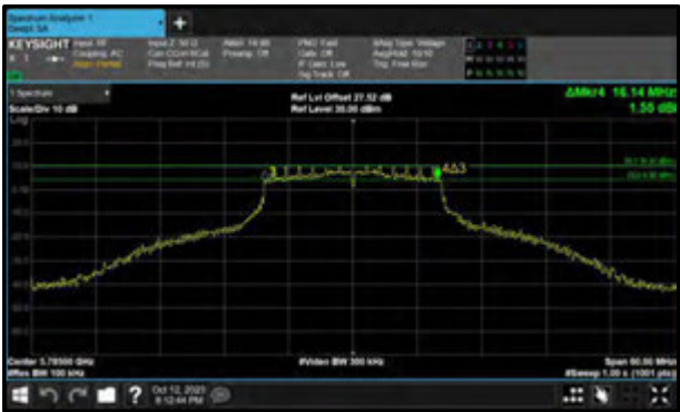
Figure 272 - 802.11a Maximum 6 dB EBW
