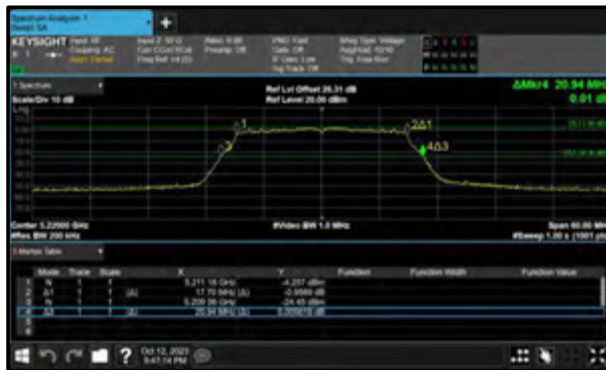
Figure 315 - 802.11n HT20 Minimum 99% OBW
