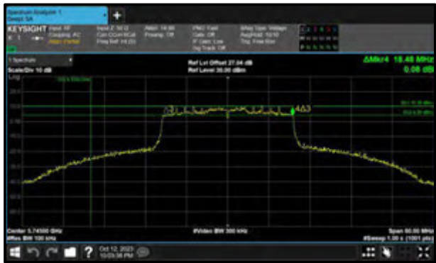
Figure 309 - 802.11ax HE20 SU Minimum 6 dB EBW
