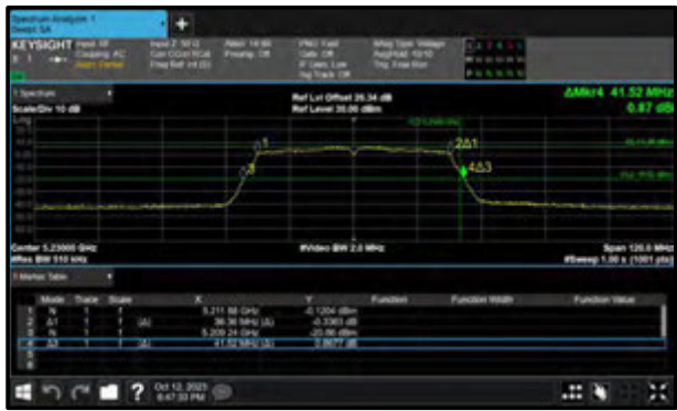
Figure 289 - 802.11n HT40 Minimum 99% OBW
