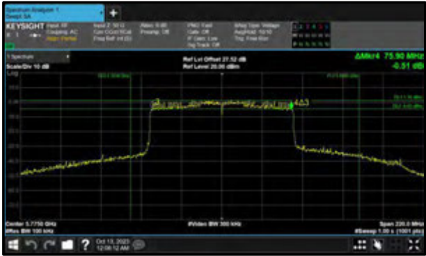
Figure 341 - 802.11ax HE80 SU Minimum 6 dB EBW
