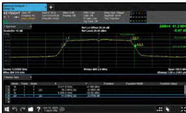
Figure 345 - 802.11n HT40 Minimum 99% OBW
