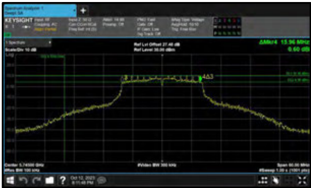
Figure 271 - 802.11a Minimum 6 dB EBW
