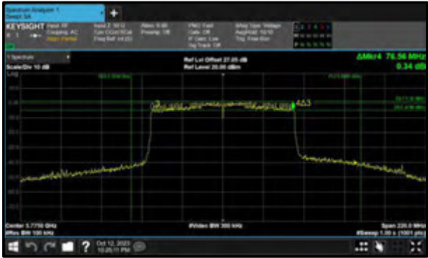
Figure 313 - 802.11ax HE80 SU Minimum 6 dB EBW
