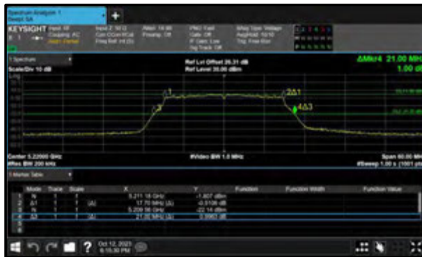
Figure 343 - 802.11n HT20 Minimum 99% OBW
