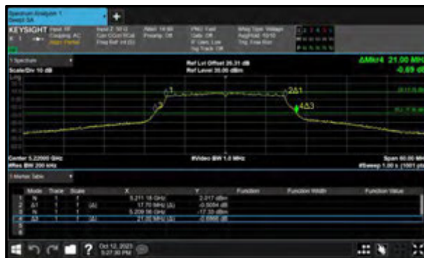
Figure 287 - 802.11n HT20 Minimum 99% OBW
