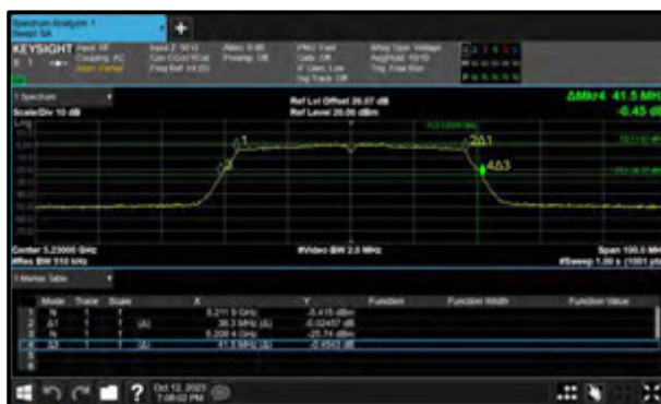
Figure 317 - 802.11n HT40 Minimum 99% OBW
