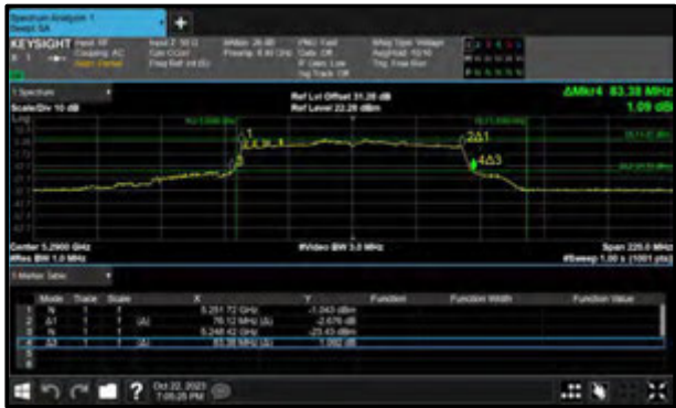
Figure 370 - 802.11ac VHT80 Maximum 99% OBW
