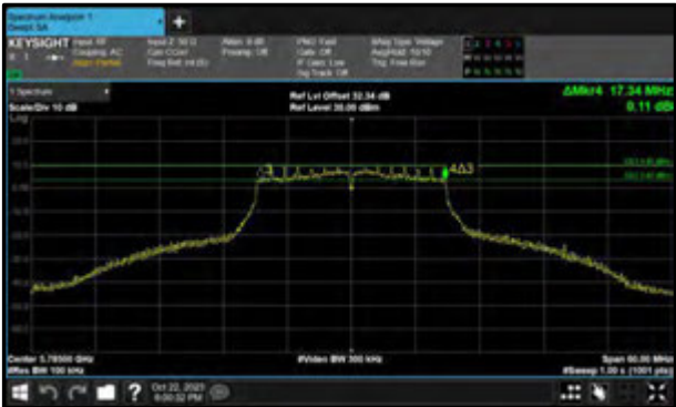
Figure 360 - 802.11ac VHT20 Maximum 6 dB EBW
