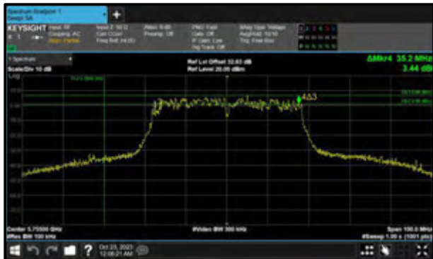
Figure 361 - 802.11ac VHT40 Minimum 6 dB EBW
