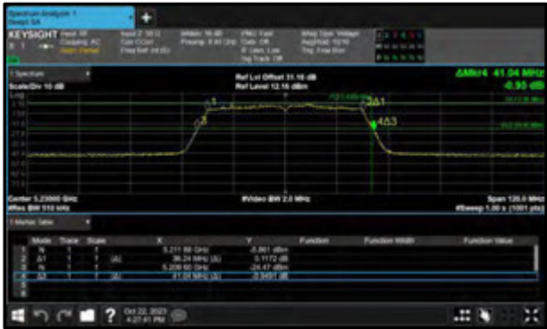
Figure 367 - 802.11ac VHT40 Minimum 99% OBW
