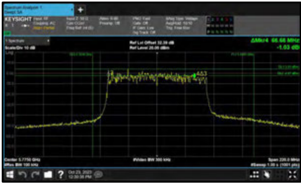
Figure 363 - 802.11ac VHT80 Minimum 6 dB EBW
