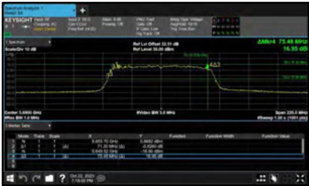
Figure 369 - 802.11ac VHT80 Minimum 99% OBW
