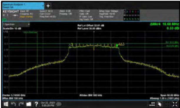
Figure 359 - 802.11ac VHT20 Minimum 6 dB EBW
