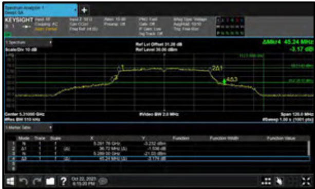
Figure 368 - 802.11ac VHT40 Maximum 99% OBW
