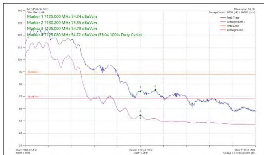
Figure 127 - 802.11ax HE20, RU 106-53, SDM, Core 0 + Core 1 - 7095 MHz Band Edge Frequency 7125 MHz
