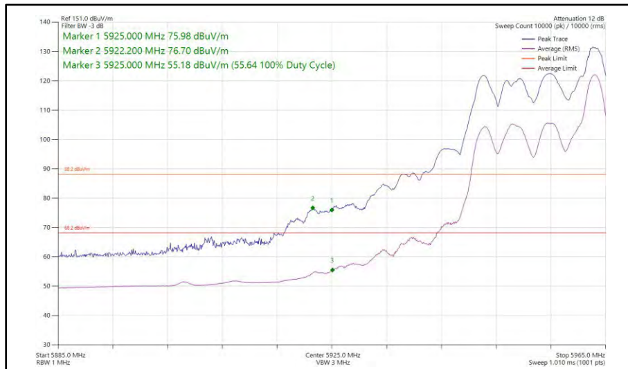
Figure 125 - 802.11ax HE20, RU 26-8, SDM, Core 0 + Core 1 - 5955 MHz Band Edge Frequency 5925 MHz
