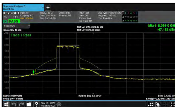
Figure 251 - A (Core 0) 802.11ax HE160 SU SP 6345 MHz (CH79)
