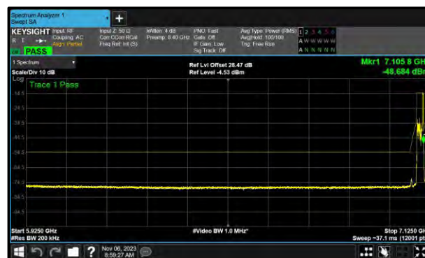
Figure 245 - A (Core 0) 802.11ax HE20 RU26 LPI 7095 MHz (CH229)
