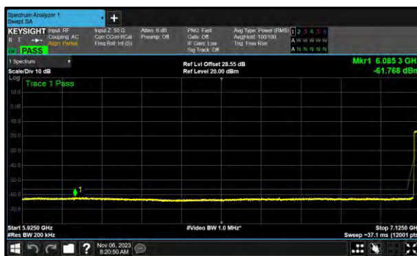
Figure 239 - A (Core 0) 802.11a LPI 7115 MHz (CH233)
