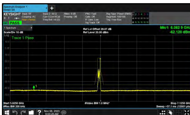
Figure 246 - B (Core 1) 802.11ax HE20 RU52 LPI 6515 MHz (CH113)
