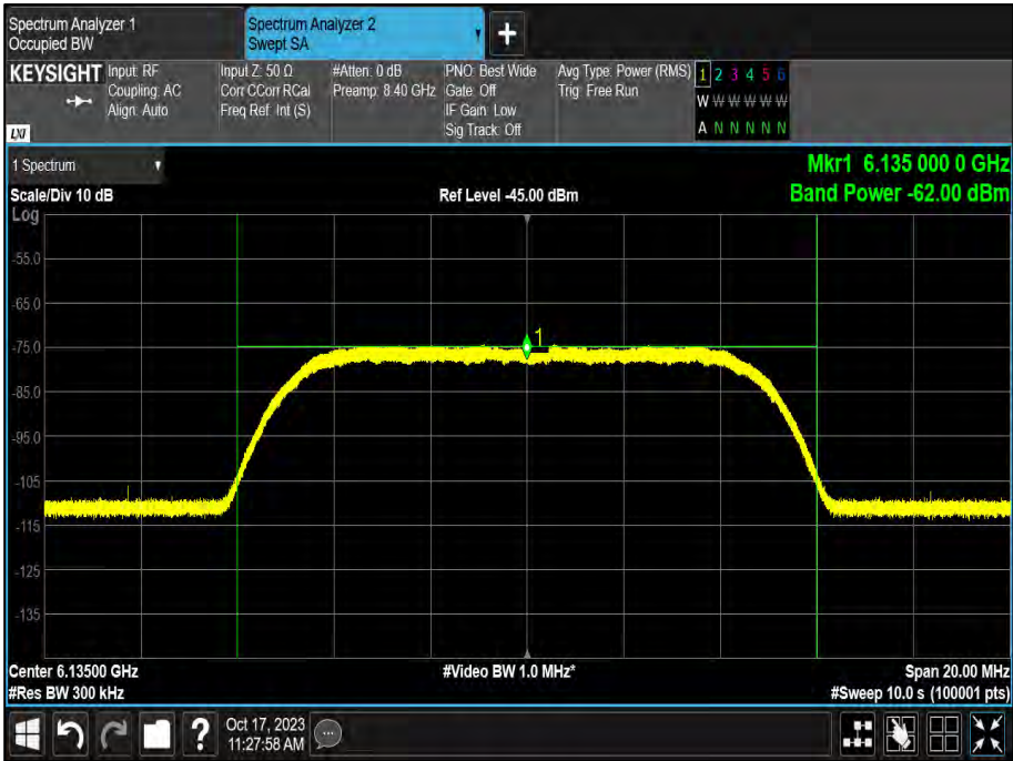
Figure 288 - Example of AWGN Signal
