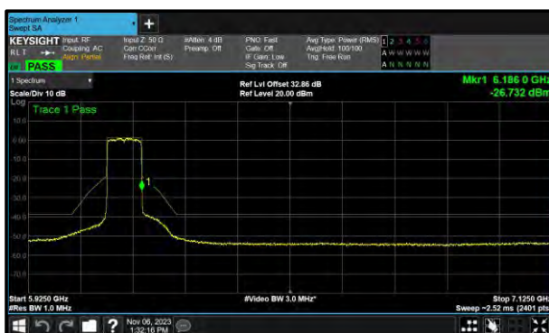
Figure 286 - A (Core 0) 802.11ax HE80 SU SP 6145 MHz (CH39)
