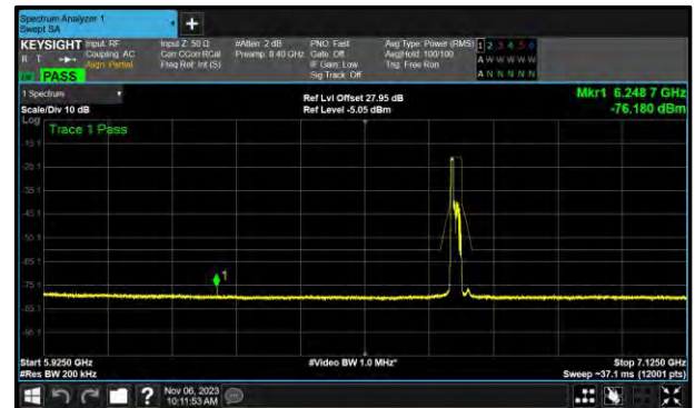
Figure 260 - B (Core 1) 802.11ax HE20 RU52 LPI 6695 MHz (CH149)
