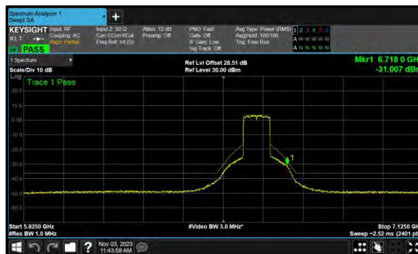
Figure 277 - A (Core 0) 802.11ax HE80 SU SP 6625 MHz (CH135)
