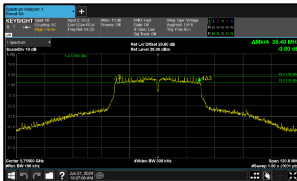
Figure 249 - 802.11n HT40 Minimum 6 dB EBW
