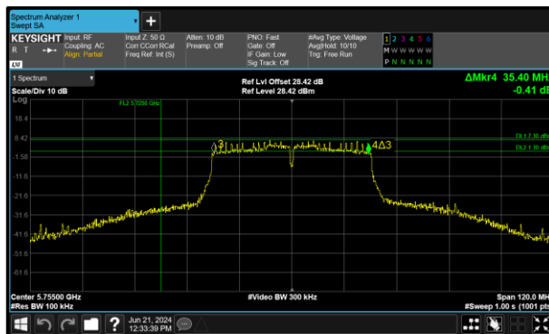
Figure 277 - 802.11n HT40 Minimum 6 dB EBW
