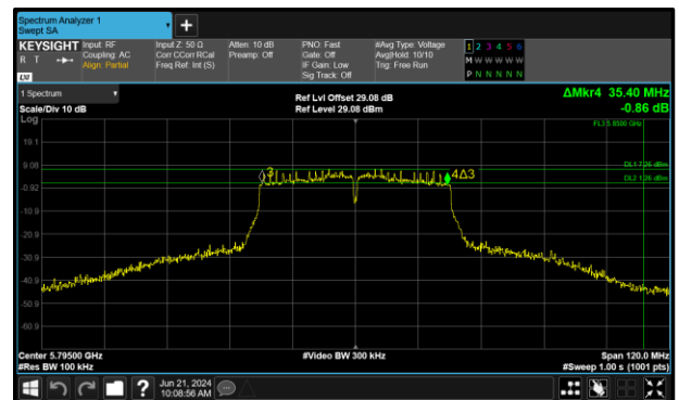
Figure 250 - 802.11n HT40 Maximum 6 dB EBW
