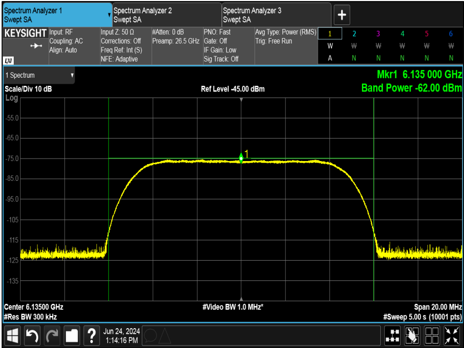
Figure 360 - Example of AWGN Signal
