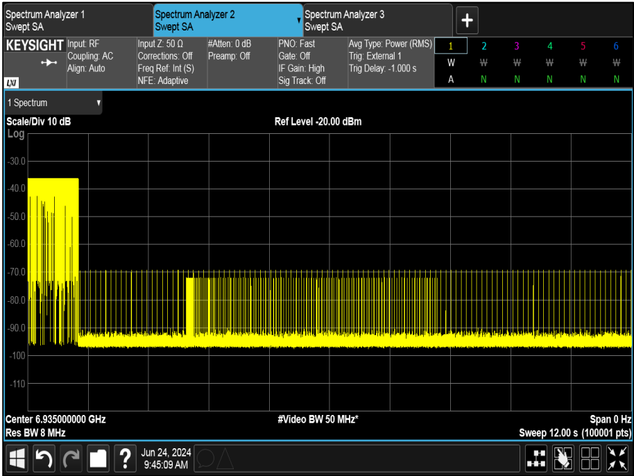
Figure 460 - U-NII-8, Minimum Bandwidth (AWGN Low)
