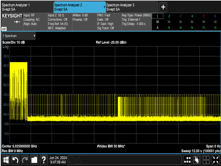
Figure 461 - U-NII-8, Minimum Bandwidth (AWGN Mid)
