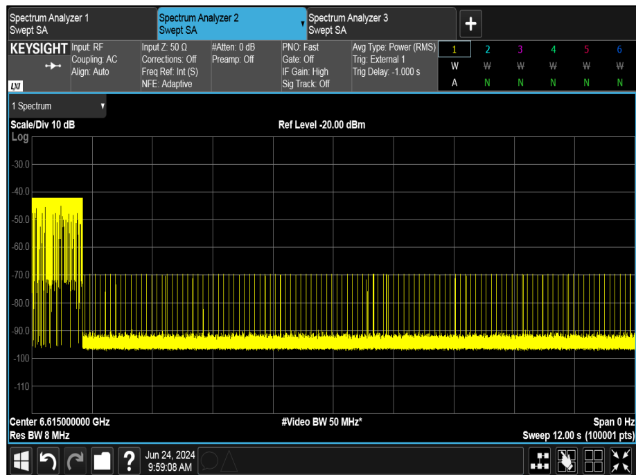
Figure 458 - U-NII-7, Minimum Bandwidth (AWGN High)
