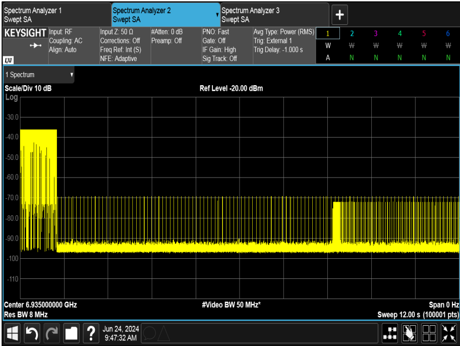
Figure 462 - U-NII-8, Minimum Bandwidth (AWGN High)
