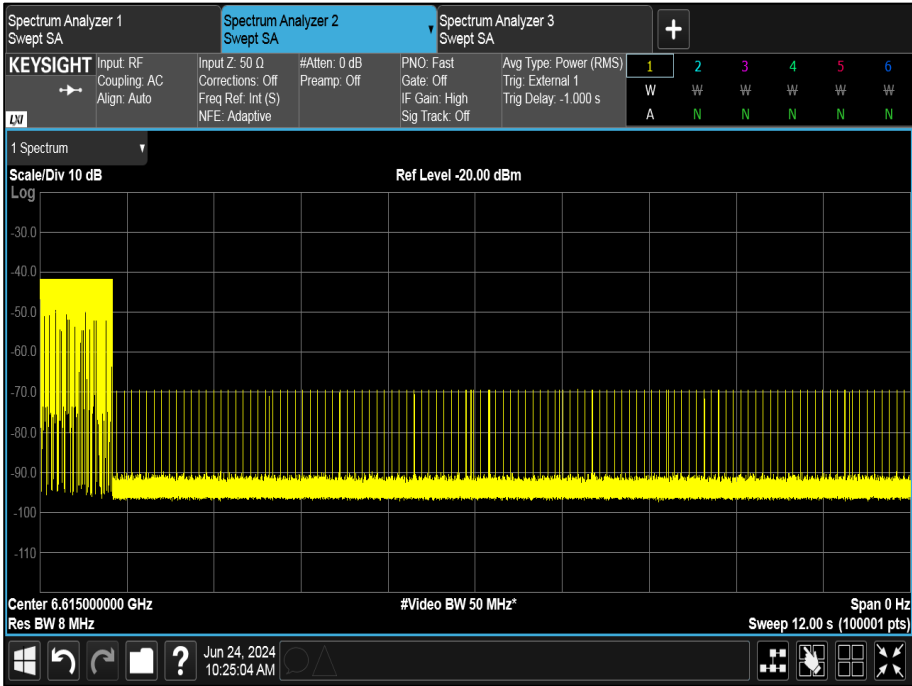
Figure 457 - U-NII-7, Minimum Bandwidth (AWGN Mid)
