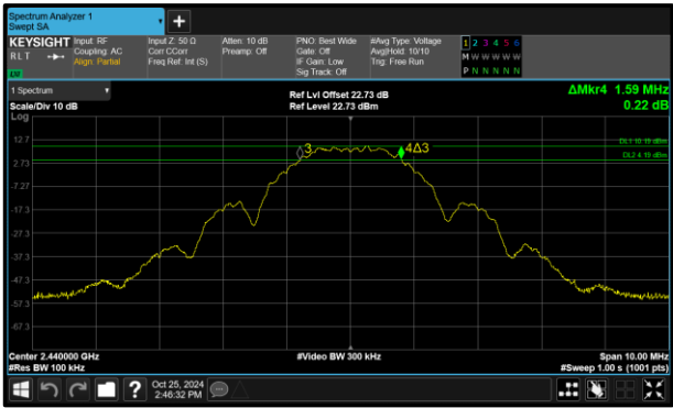
Figure 14 - Core 0 (A) 2440 MHz (CH18) 6 dB Bandwidth
