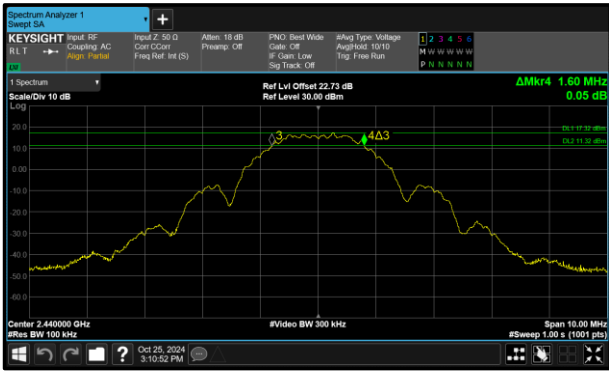
Figure 20 - Core 0 (A) 2440 MHz (CH18) 6 dB Bandwidth
