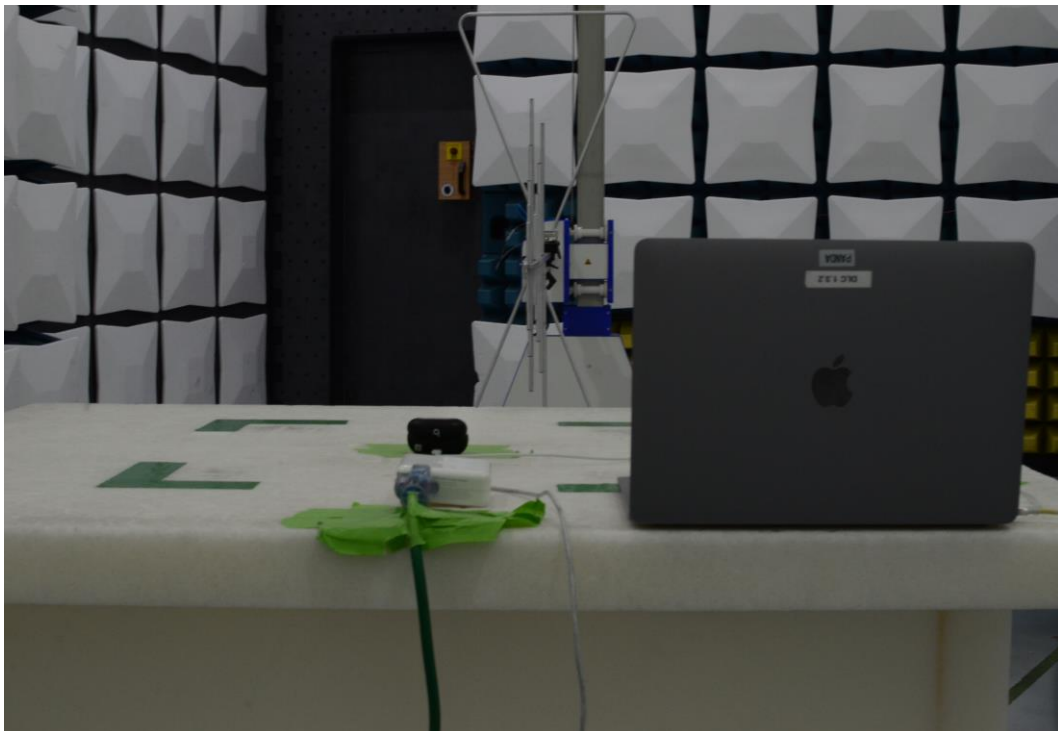
Figure 16: 30MHz-1GHz Test Setup (Rear View)
