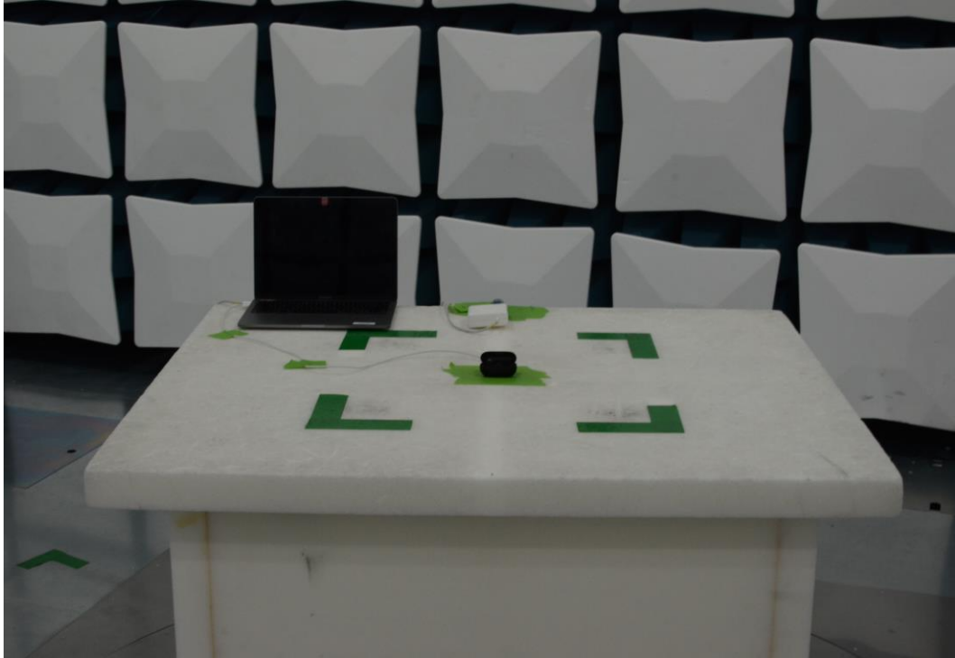
Figure 15: 30MHz-1GHz Test Setup (Front View)
