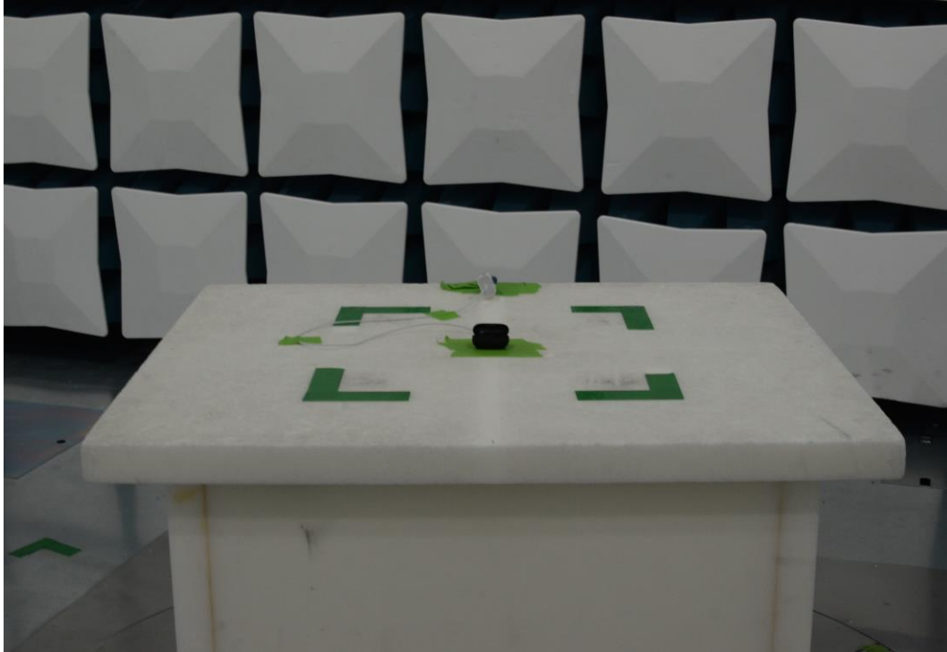
Figure 13: 30MHz-1GHz Test Setup (Front View)
