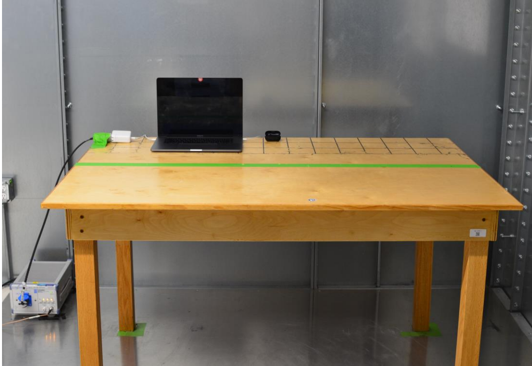
Figure 3: AC Line Conducted Emissions (Front View)
