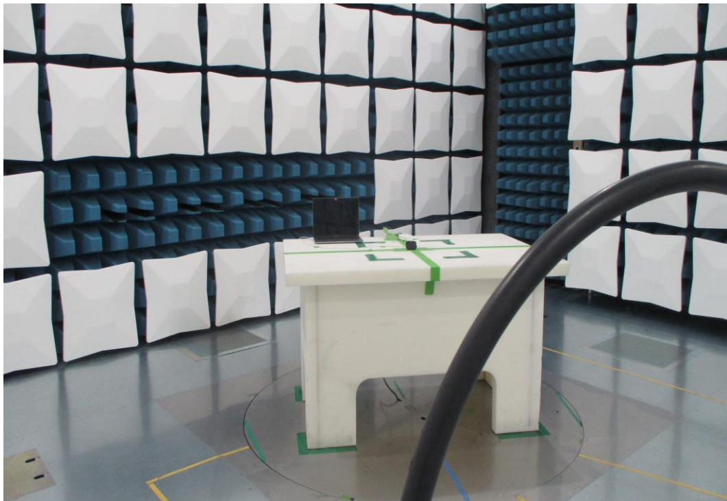
Figure 18: 9kHz-30MHz Test Setup (Front View)
