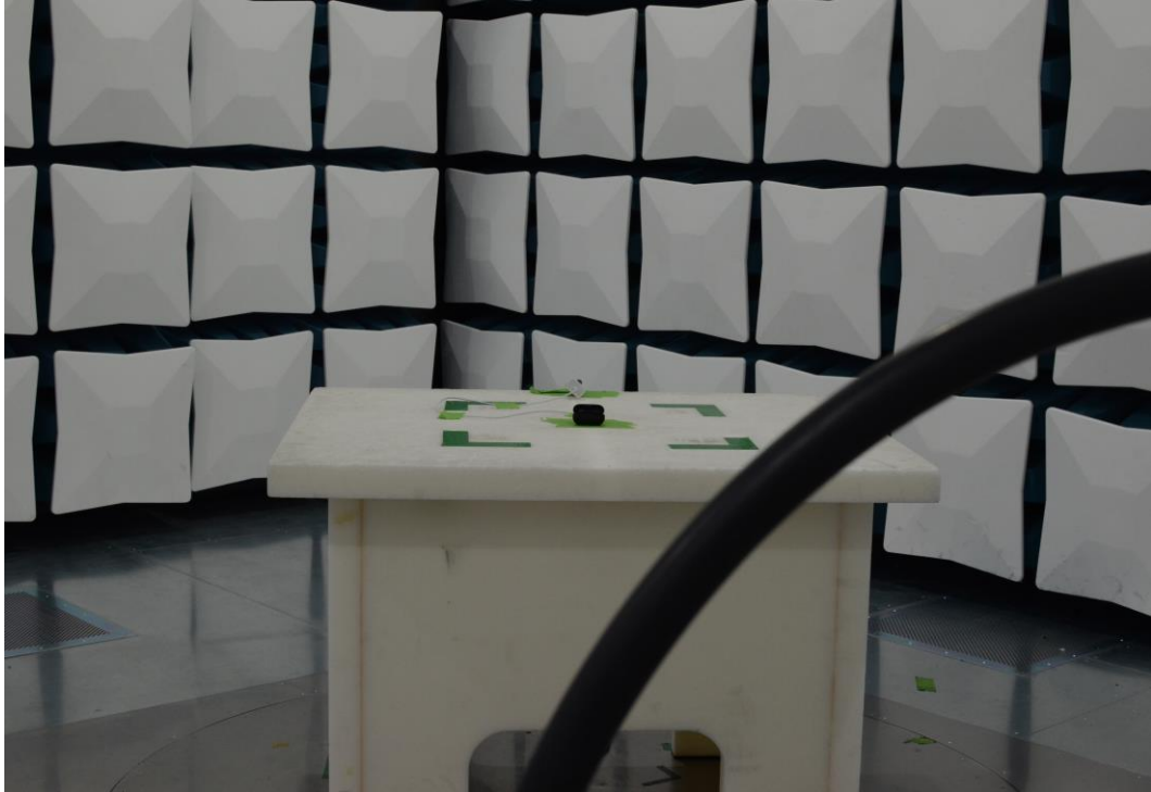
Figure 17: 9kHz-30MHz Test Setup (Front View)
