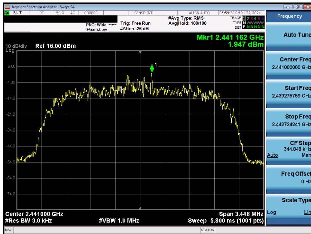
Plot 7-14. Power Spectral Density Plot (Bluetooth (HDR4), 4Mbps, – Ch. 38)
