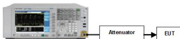
Figure 7-3. Test Instrument & Measurement Setup
