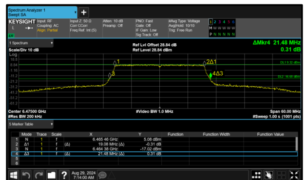
Figure 114 - 802.11ax HE20 SU SP Maximum 26 dB EBW
