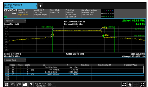
Figure 118 - 802.11ax HE80 SU SP Maximum 26 dB EBW
