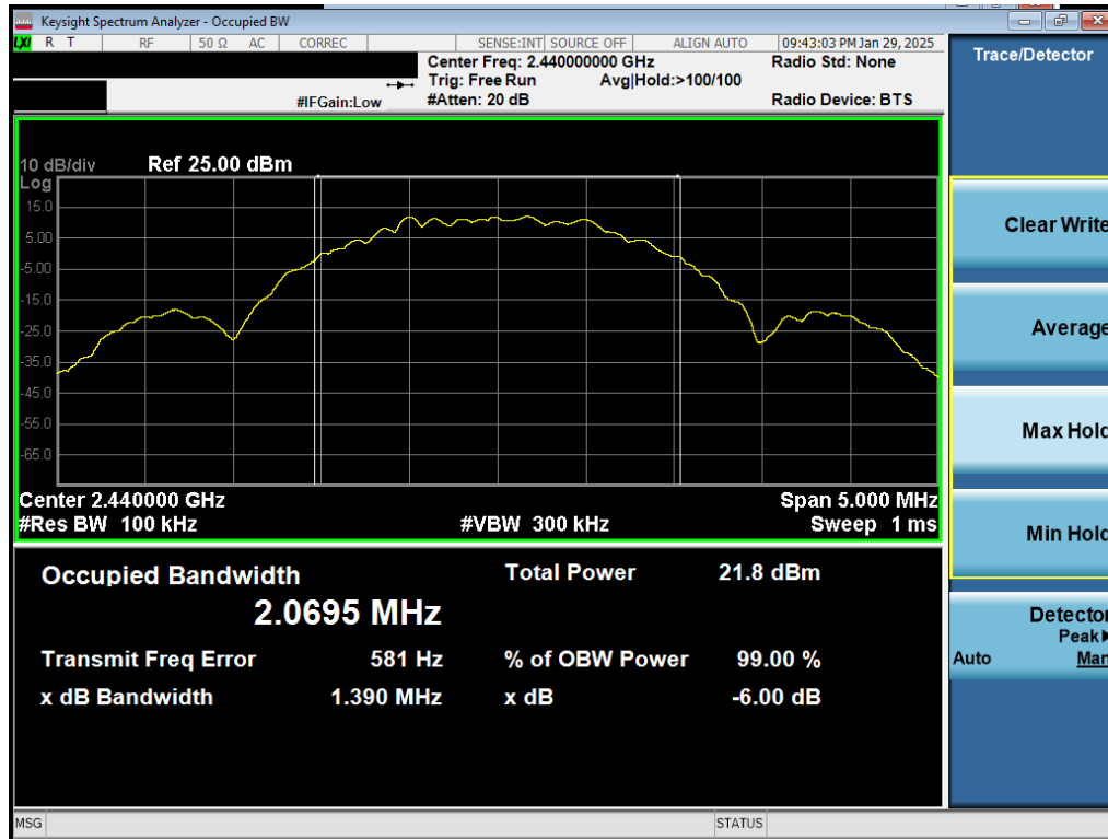
Plot 7-23. 6dB BW Plot Antenna 0 (Dedicated) (Bluetooth (LE), 2Mbps, iPA – Ch. 19)
