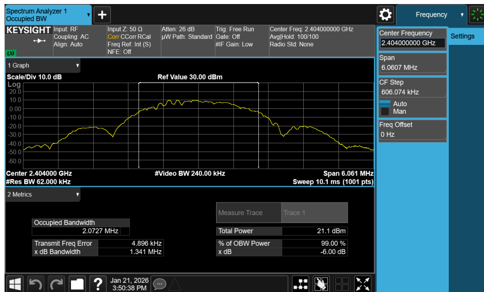
Plot 7-4. 99% OBW Plot Antenna 0 (Common) (Bluetooth (LE), 2Mbps, iPA – Ch. 1)
