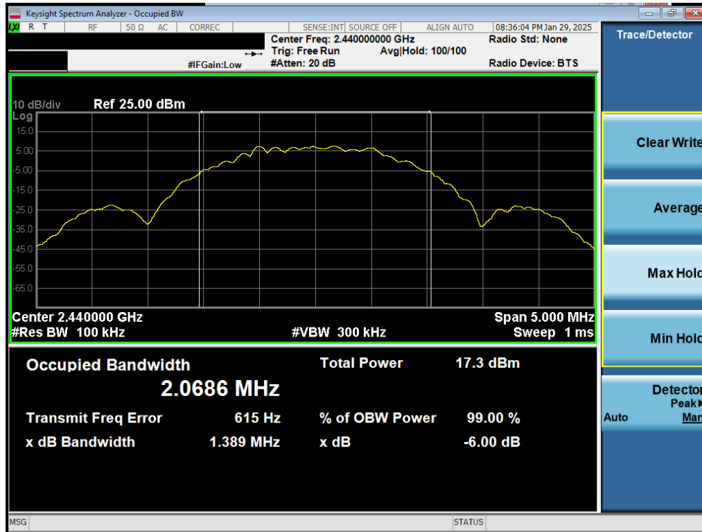
Plot 7-17. 6dB BW Plot Antenna 0 (Common) (Bluetooth (LE), 2Mbps, iPA – Ch. 19)
