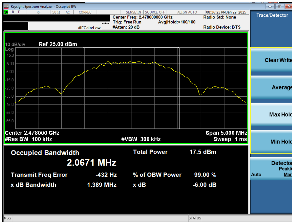
Plot 7-18. 6dB BW Plot Antenna 0 (Common) (Bluetooth (LE), 2Mbps, iPA – Ch. 38)
