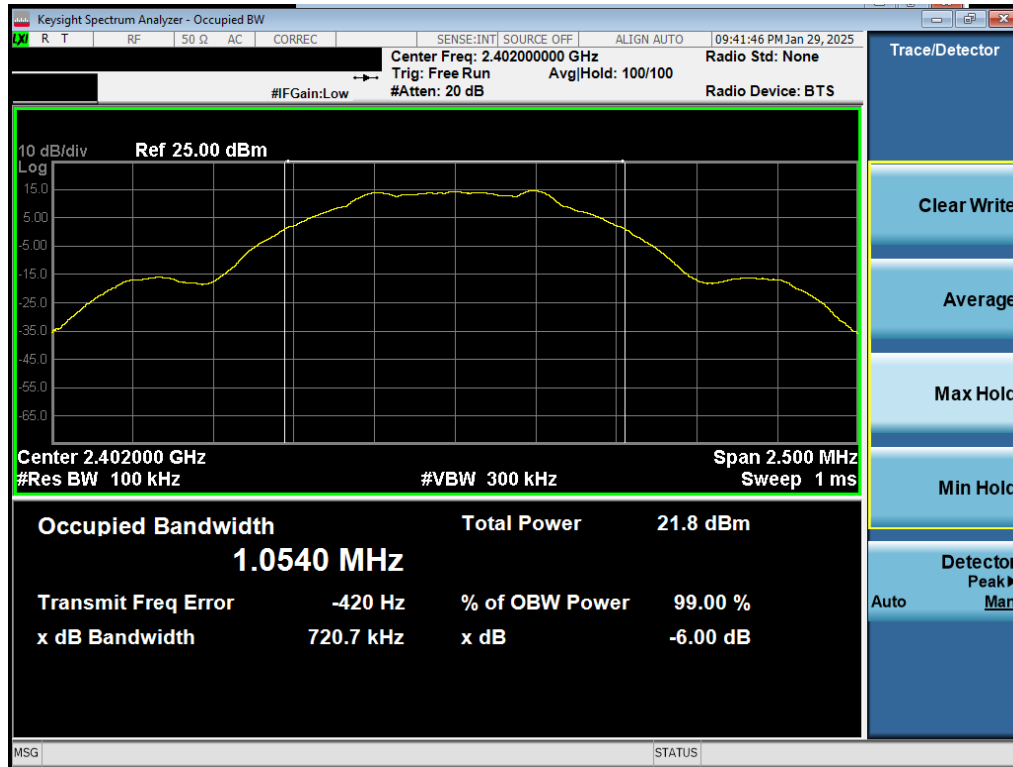
Plot 7-19. 6dB BW Plot Antenna 0 (Dedicated) (Bluetooth (LE), 1Mbps, iPA – Ch. 0)
