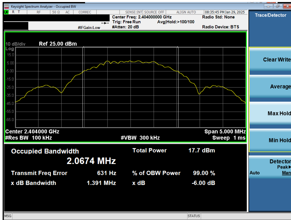
Plot 7-16. 6dB BW Plot Antenna 0 (Common) (Bluetooth (LE), 2Mbps, iPA – Ch. 1)
