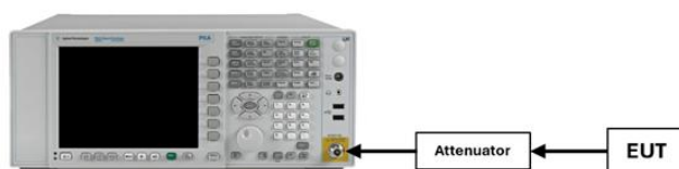
Figure 7-5. Test Instrument & Measurement Setup
