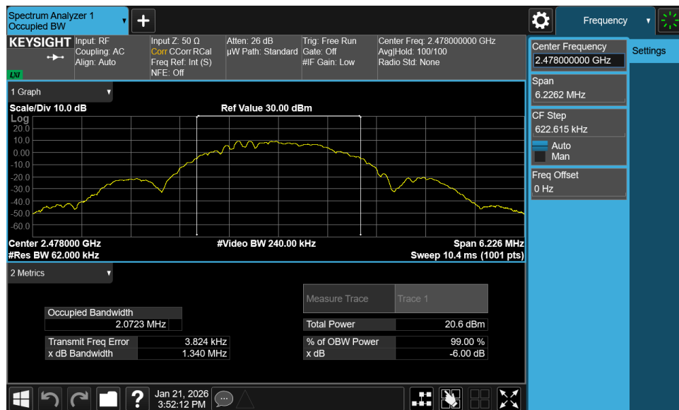
Plot 7-6. 99% OBW Plot Antenna 0 (Common) (Bluetooth (LE), 2Mbps, iPA – Ch. 38)
