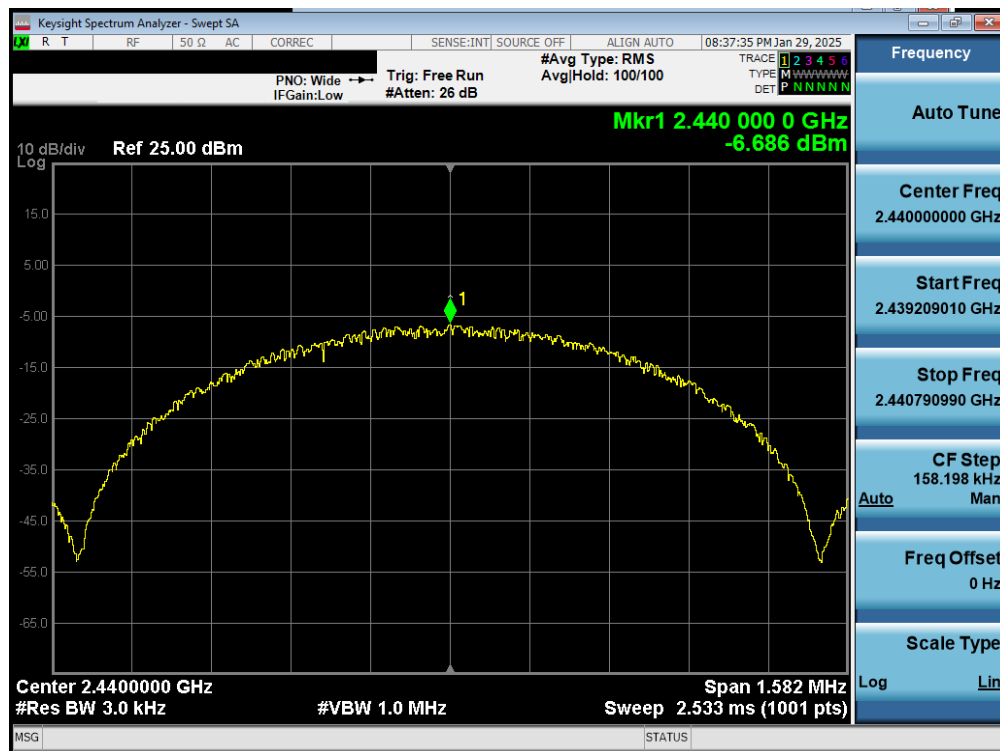
Plot 7-26. Power Spectral Density Plot Antenna 0 (Common) (Bluetooth (LE), 1Mbps, iPA – Ch. 19)
