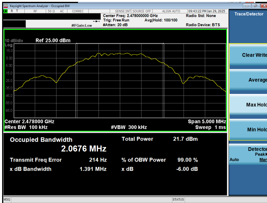
Plot 7-24. 6dB BW Plot Antenna 0 (Dedicated) (Bluetooth (LE), 2Mbps, iPA – Ch. 38)
