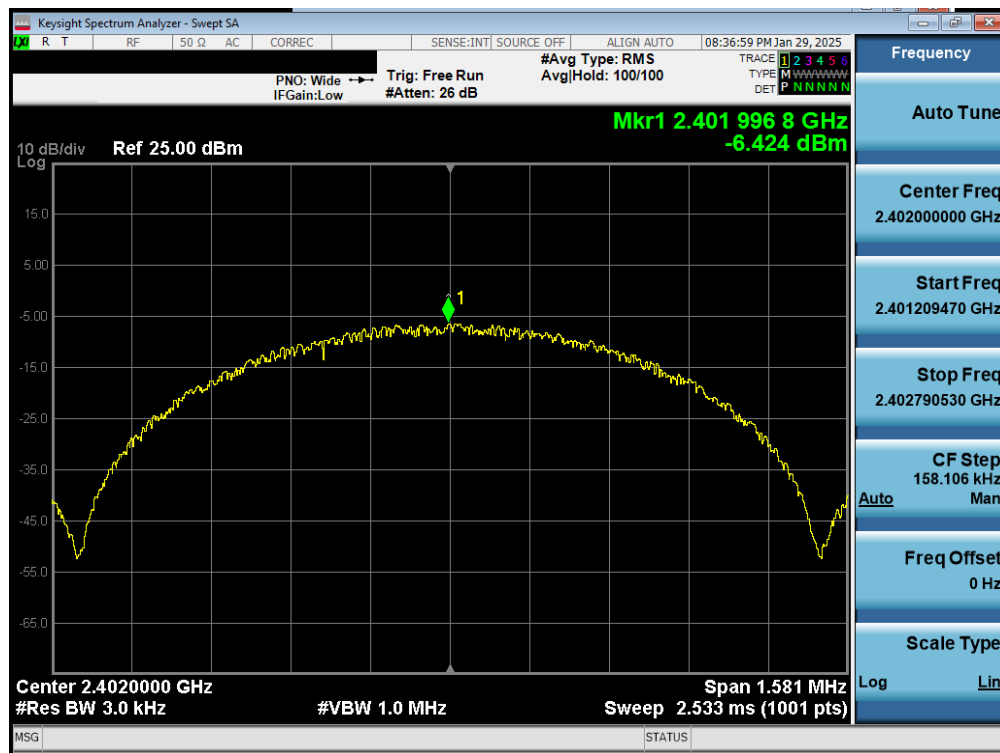
Plot 7-25. Power Spectral Density Plot Antenna 0 (Common) (Bluetooth (LE), 1Mbps, iPA – Ch. 0)
