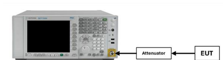
Figure 7-6. Test Instrument & Measurement Setup
