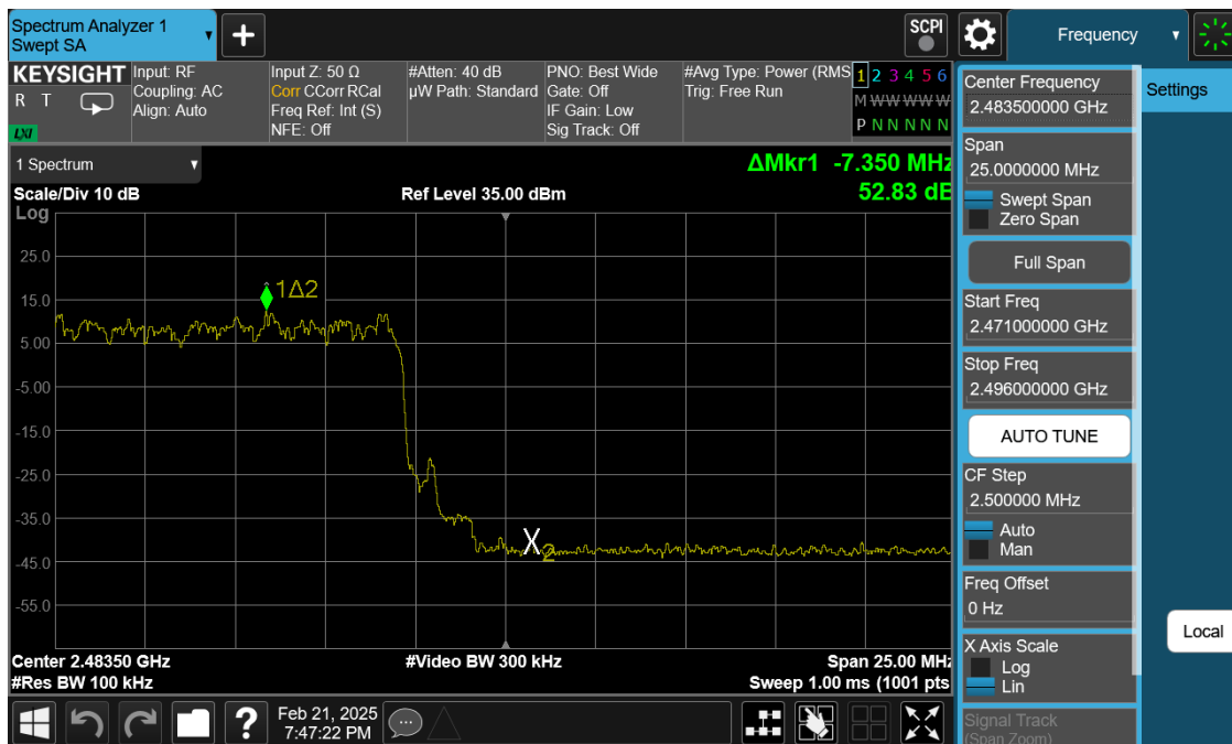
Plot 7-20. Band Edge Plot Antenna 0 (Common) (Bluetooth with Hopping Enabled, 8DPSK, iPA – Ch. 78)
