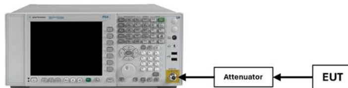
Figure 7-3. Test Instrument & Measurement Setup
