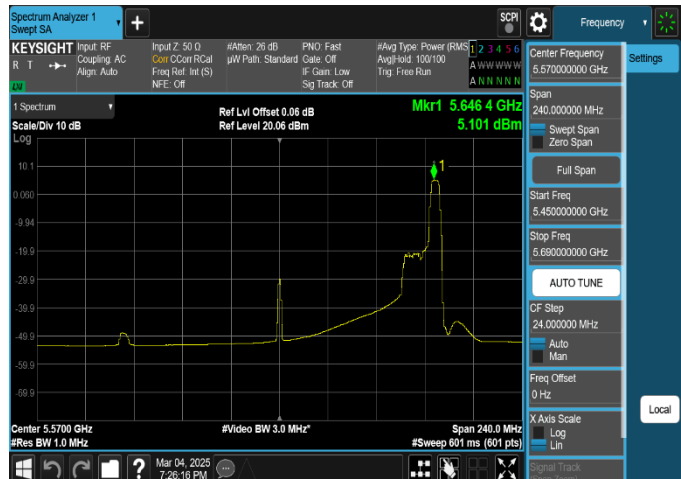
Plot 7-52. (FCC Only) PSD Antenna 1 (160MHz BW 11ax Index52 – RU52 – Ch.114)
