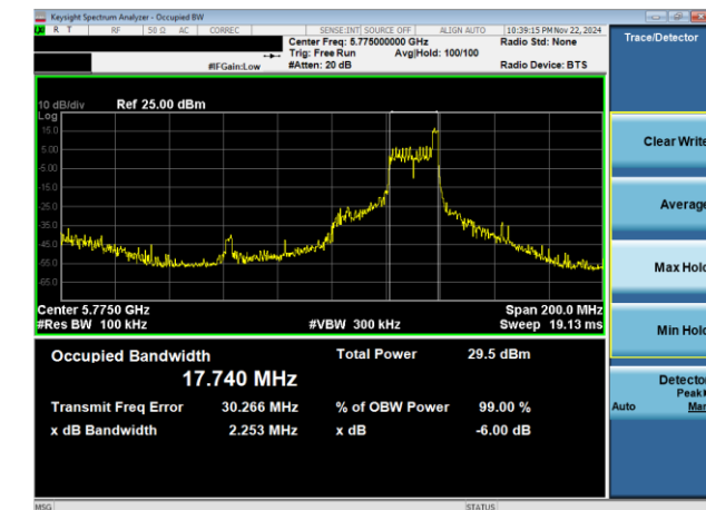
Plot 7-19. 6dB BW OBW Antenna 0 (80MHz BW 11ax Index 36 – RU26 – Ch.155)
