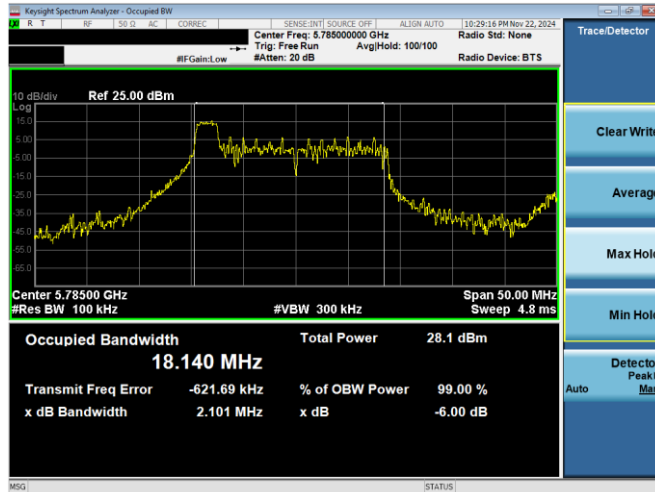
Plot 7-17. 6dB BW OBW Antenna 0 (20MHz BW 11ax Index 0 – RU26 – Ch.157)
