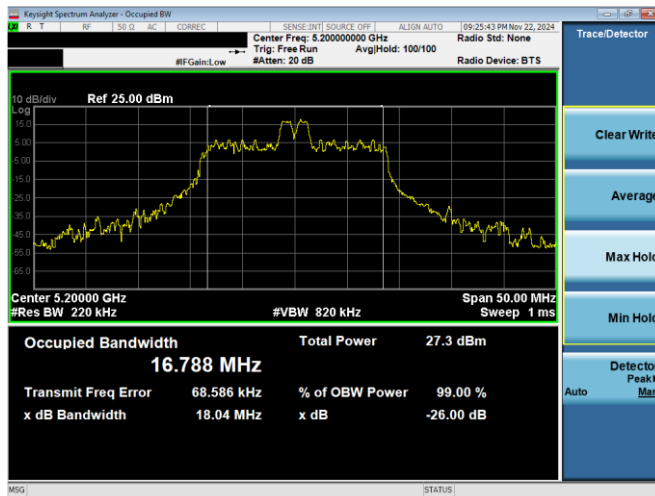
Plot 7-1. 26dB BW & 99% OBW Antenna 0 (20MHz BW 11ax Index 4 – RU26 – Ch.40)
