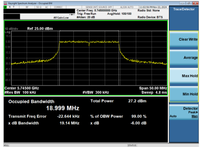
Plot 7-20. 6dB BW OBW Antenna 0 (20MHz BW 11ax– RU242 – Ch.149)
