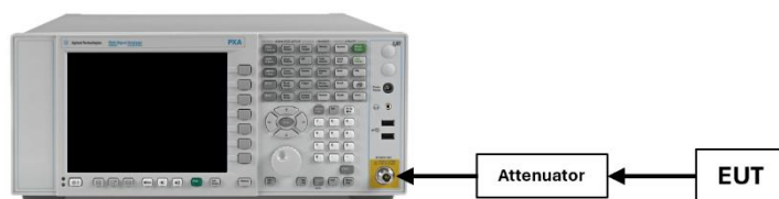
Figure 7-1. Test Instrument & Measurement Setup
