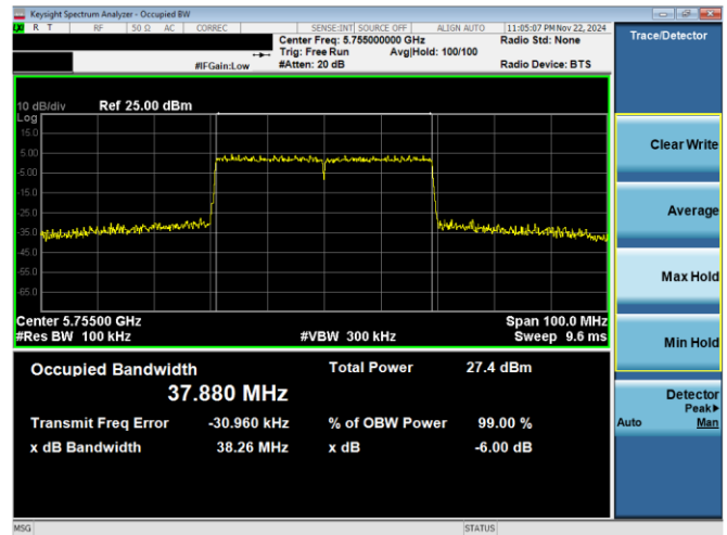
Plot 7-21. 6dB BW OBW Antenna 0 (40MHz BW 11ax– RU484 – Ch.151)
