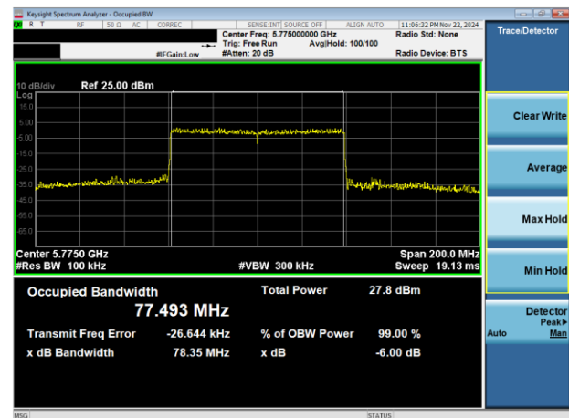
Plot 7-22. 6dB BW OBW Antenna 0 (80MHz BW 11ax– RU996 – Ch.155)
