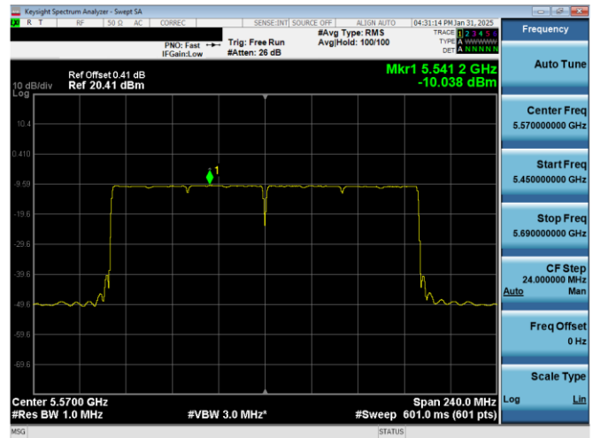
Plot 7-36. PSD Antenna 0 (160MHz BW 11ax- RU996x2 - Ch.114
