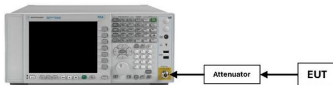
Figure 7-4. Test Instrument & Measurement Setup
