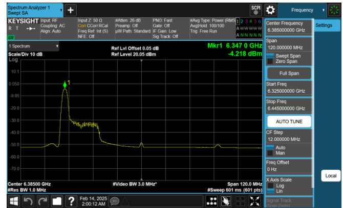
Plot 7-139. PSD Plot Antenna 0 (80MHz 802.11ax RU26 (UNII Band 5) – Ch. 87)
