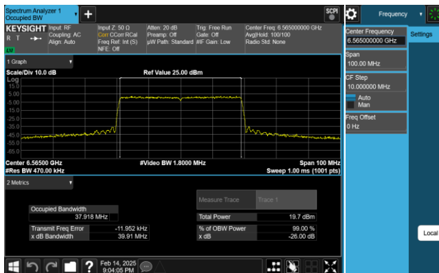
Plot 7-102. 26dB & 99% Bandwidth Plot Antenna 1 (40MHz 802.11ax RU484 (UNII Band 7) – Ch. 123)
