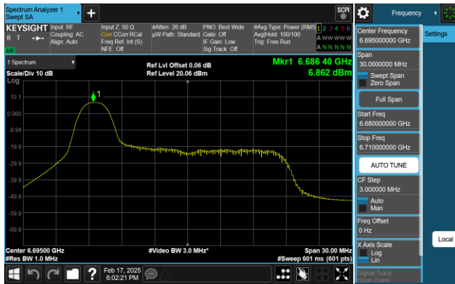
Plot 7-129. PSD Plot Antenna 0 (20MHz 802.11ax RU26 (UNII Band 7) – Ch. 149)
