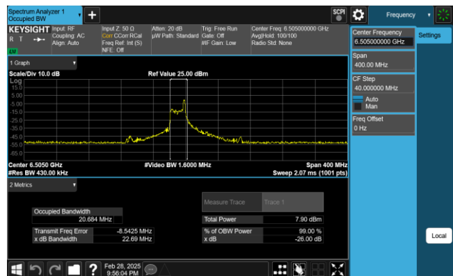
Plot 7-92. 26dB & 99% Bandwidth Plot Antenna 1 (160MHz 802.11ax RU26 (UNII Band 6) – Ch. 111)
