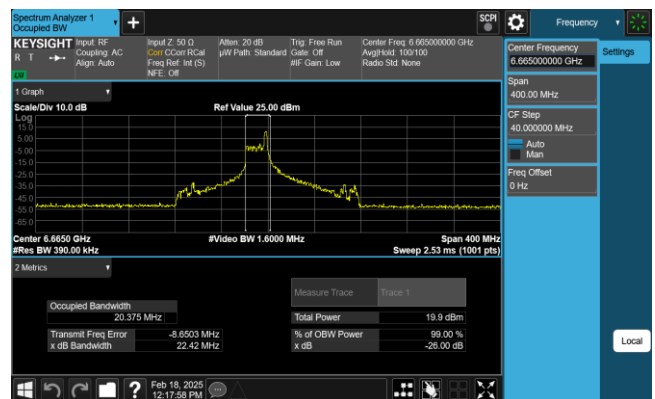
Plot 7-76. 26dB & 99% Bandwidth Plot Antenna 1 (160MHz 802.11ax RU26 (UNII Band 7) – Ch. 143)
