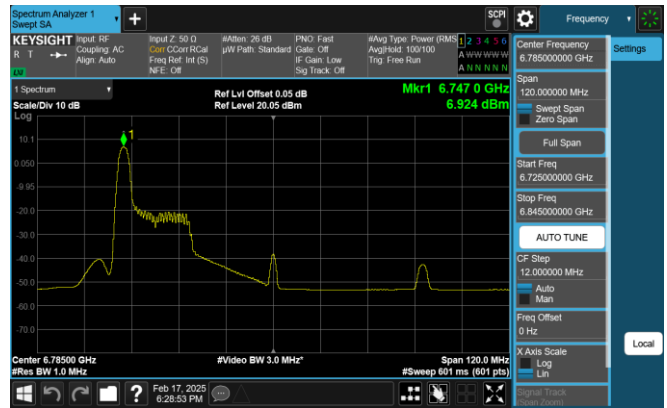
Plot 7-131. PSD Plot Antenna 0 (80MHz 802.11ax RU26 (UNII Band 7) – Ch. 167)
