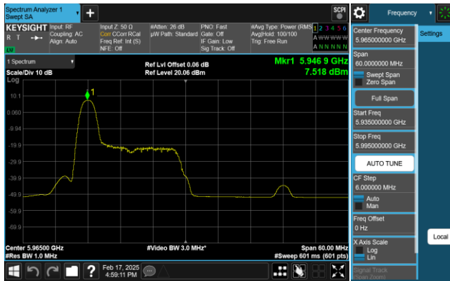
Plot 7-114. PSD Plot Antenna 0 (40MHz 802.11ax RU26 (UNII Band 5) – Ch. 3)
