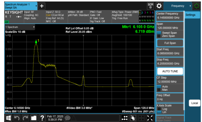
Plot 7-115. PSD Plot Antenna 0 (80MHz 802.11ax RU26 (UNII Band 5) – Ch. 39)
