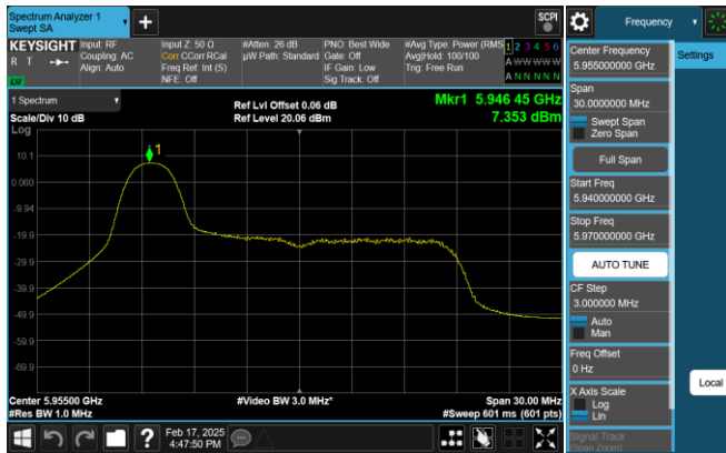
Plot 7-113. PSD Plot Antenna 0 (20MHz 802.11ax RU26 (UNII Band 5) – Ch. 1)
