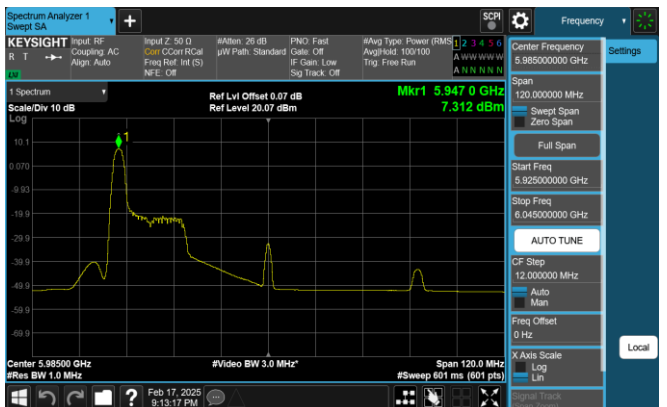
Plot 7-229. PSD Plot SDM Antenna 0 (80MHz 802.11ax RU26 (Ulll Band 5) – Ch. 7)
