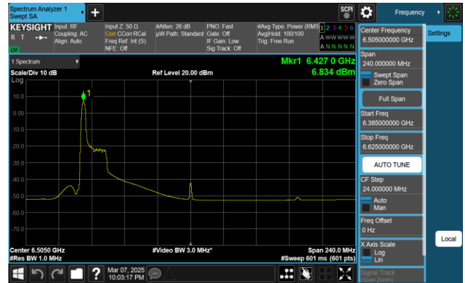
Plot 7-248. PSD Plot SDM Antenna 0 (160MHz 802.11ax RU26 (UNII Band 6) - Ch. 111)
