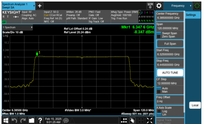
Plot 7-286. PSD Plot SDM Antenna 1 (80MHz 802.11ax RU996 (UNII Band 5) - Ch. 87)
