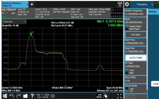
Plot 7-259. PSD Plot SDM Antenna 0 (40MHz 802.11ax RU26 (U-NII Band 7) - Ch. 155)
