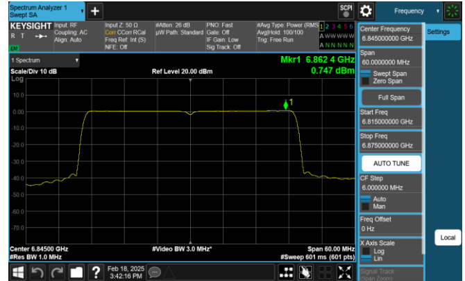
Plot 7-268. PSD Plot CDD Antenna 0 (40MHz 802.11ax RU484 (UNII Band 7) - Ch. 179)
