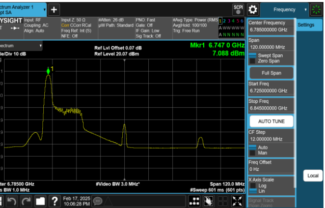
Plot 7-261. PSD Plot SDM Antenna 0 (80MHz 802.11ax RU26 (U-NII Band 7) - Ch. 167)
