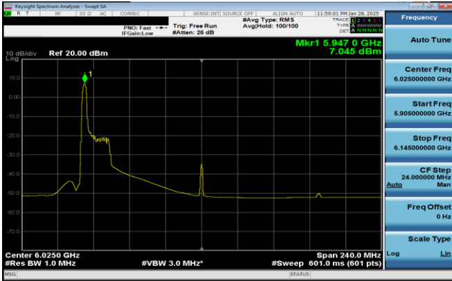
Plot 7-232. PSD Plot SDM Antenna 1 (160MHz 802.11ax RU26 (UNII Band 5) – Ch. 15)
