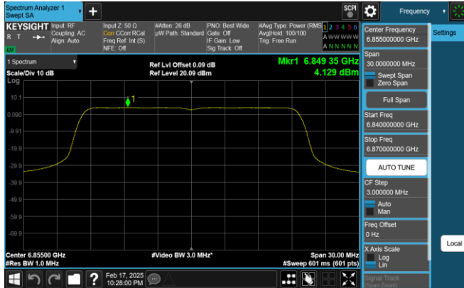
Plot 7-265. PSD Plot SDM Antenna 0 (20MHz 802.11ax RU242 (UNII Band 7) - Ch. 181)
