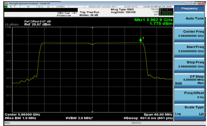
Plot 7-236. PSD Plot SDM Antenna 1 (40MHz 802.11ax RU484 (UNII Band 5) - Ch. 3)
