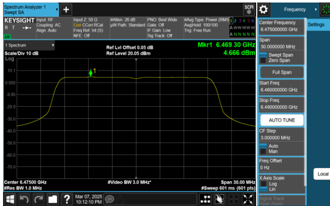
Plot 7-250. PSD Plot SDM Antenna 0 (20MHz 802.11ax RU242 (UNII Band 6) - Ch. 105)
