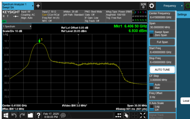
Plot 7-225. PSD Plot SDM Antenna 0 (20MHz 802.11ax RU26 (Ulll Band 5) – Ch. 93)
