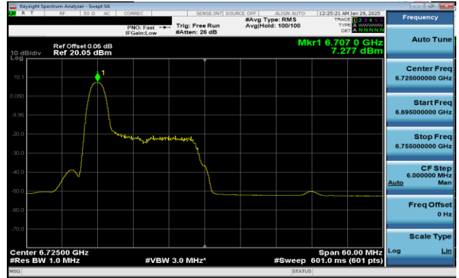
Plot 7-260. PSD Plot SDM Antenna 0 (40MHz 802.11ax RU26 (U-NII Band 7) - Ch. 155)
