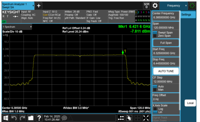
Plot 7-285. PSD Plot SDM Antenna 0 (80MHz 802.11ax RU996 (UNII Band 5) - Ch. 87)
