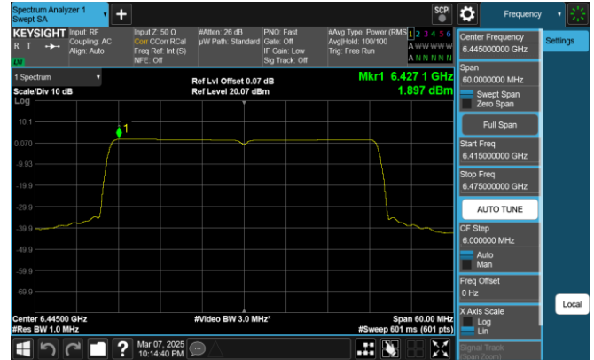
Plot 7-252. PSD Plot CDD Antenna 0 (40MHz 802.11ax RU484 (UNII Band 6) - Ch. 99)
