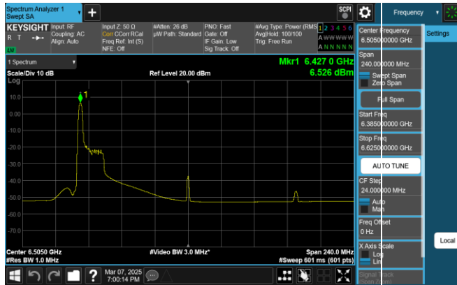
Plot 7-247. PSD Plot SDM Antenna 0 (160MHz 802.11ax RU26 (UNII Band 6) - Ch. 111)
