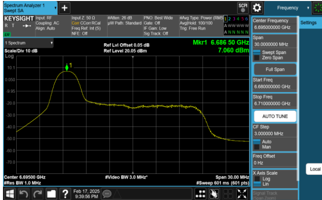
Plot 7-257. PSD Plot SDM Antenna 0 (20MHz 802.11ax RU26 (U-NII Band 7) - Ch. 149)
