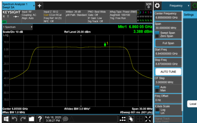
Plot 7-266. PSD Plot SDM Antenna 0 (20MHz 802.11ax RU242 (UNII Band 7) - Ch. 181)
