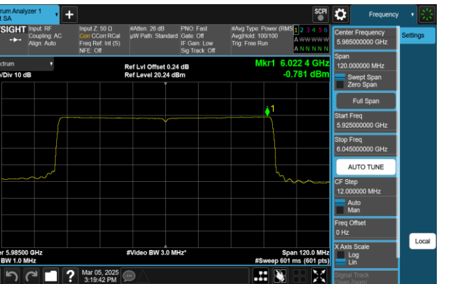
Plot 7-237. PSD Plot CDD Antenna 0 (80MHz 802.11ax RU996 (UNII Band 5) - Ch. 7)
