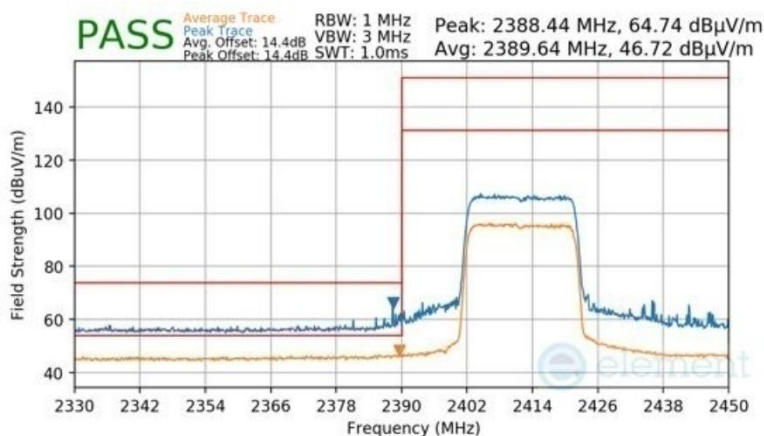
Plot 7-263 Radiated Restricted Lower Band Edge Measurement Antenna 1
