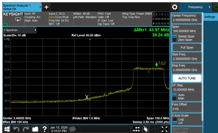
Plot 7-57. Band Edge Antenna 1 Common (802.11ax OFDMA – RU242 – Ch. 6(Low Channel))
