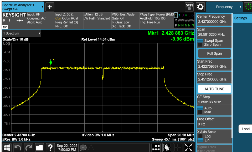
Plot 7-28. Power Spectral Density Plot Antenna 1 Dedicated (802.11ax OFDMA – RU242 – Ch. 6)
