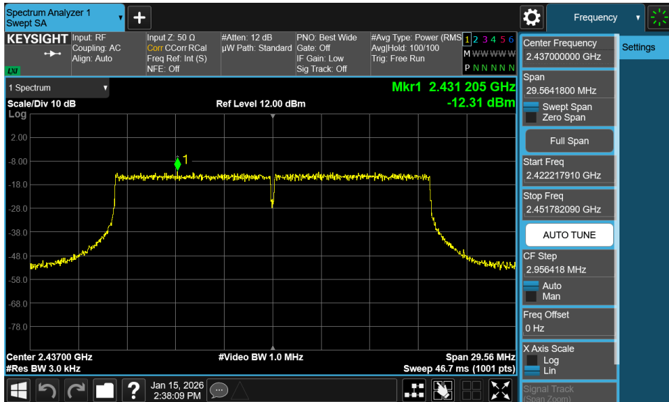
Plot 7-20. Power Spectral Density Plot Antenna 1 Common (802.11ax OFDMA – RU242 – Ch. 6)
