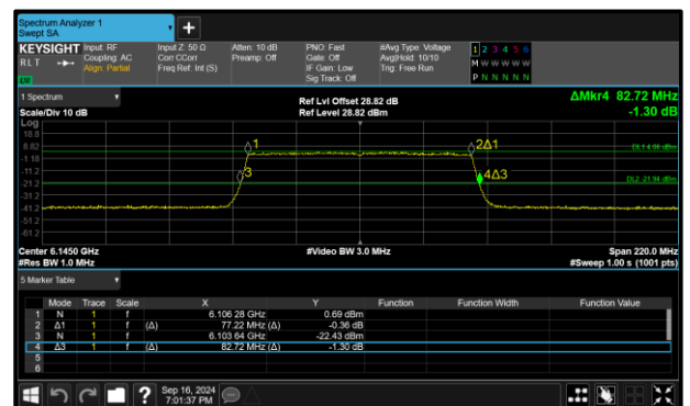
Figure 8 - 802.11ax HE80 SU LPI Maximum 26 dB EBW
