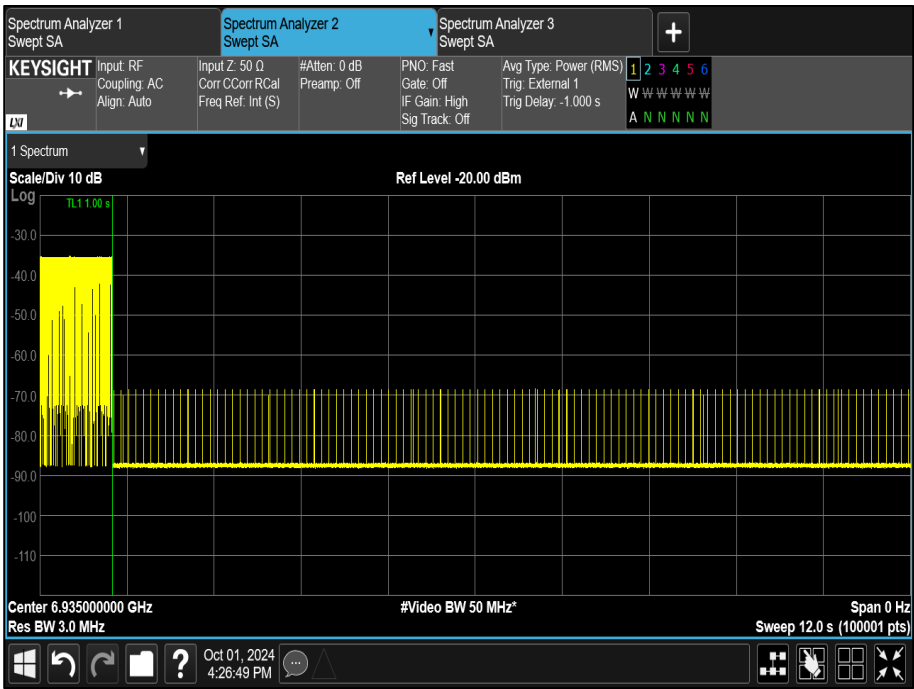
Figure 361 - U-NII-8, Maximum Bandwidth (AWGN Mid), OFF Level
