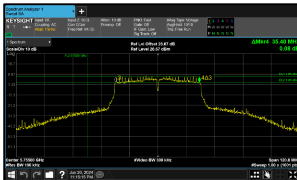
Figure 262 - 802.11n HT40 Minimum 6 dB EBW
