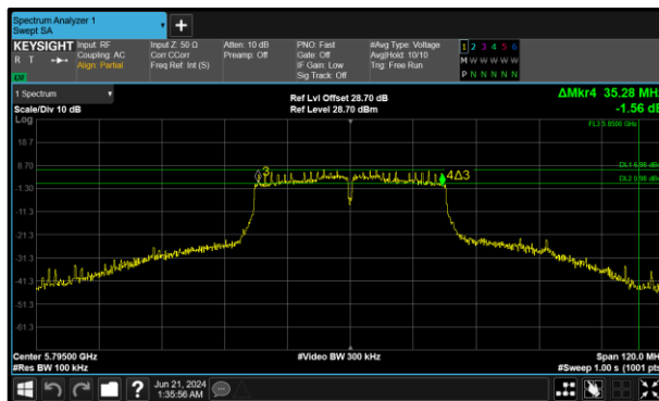
Figure 290 - 802.11n HT40 Minimum 6 dB EBW
